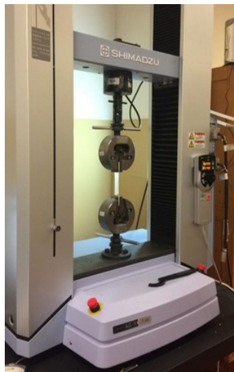
Figure 2.11: Autograph AGS-1kNX model from Shimadzu. Photo taken during the tensile tests.
