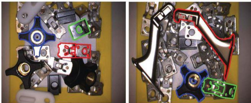
Figure 2.4- Object detection and pose estimation results from the FDCM algorithm [44].
