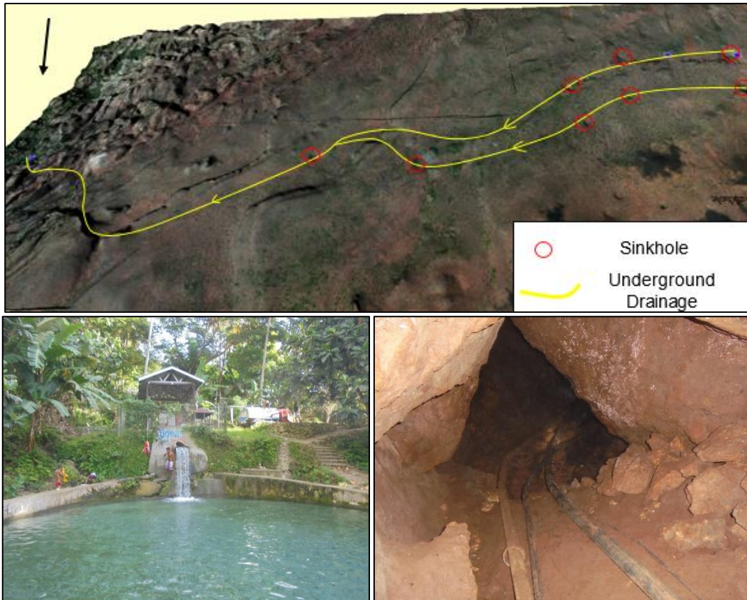
Figure 5. 12 The underground drainage pattern interpreted according to the sinkholes alignment on LIDAR and aerophoto (Top). Uailili spring (Bellow left), Uailiabere cave (Bellow right)
