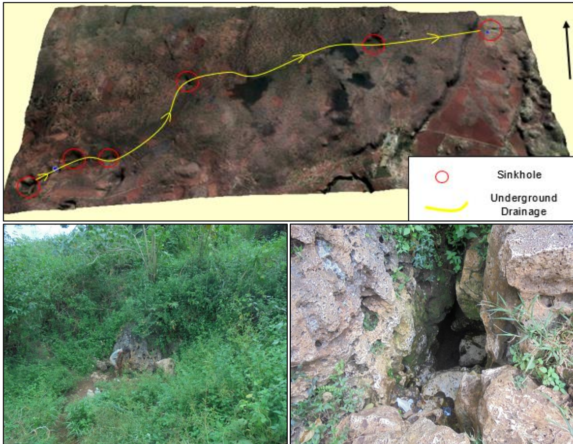
Figure 5. 11 The underground drainage pattern interpreted according to the sinkholes alignment on LIDAR and aerophoto (Top). Uaimatahun cave (Bellow)
