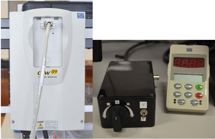
Fig. B.4. Variable speed drive.
