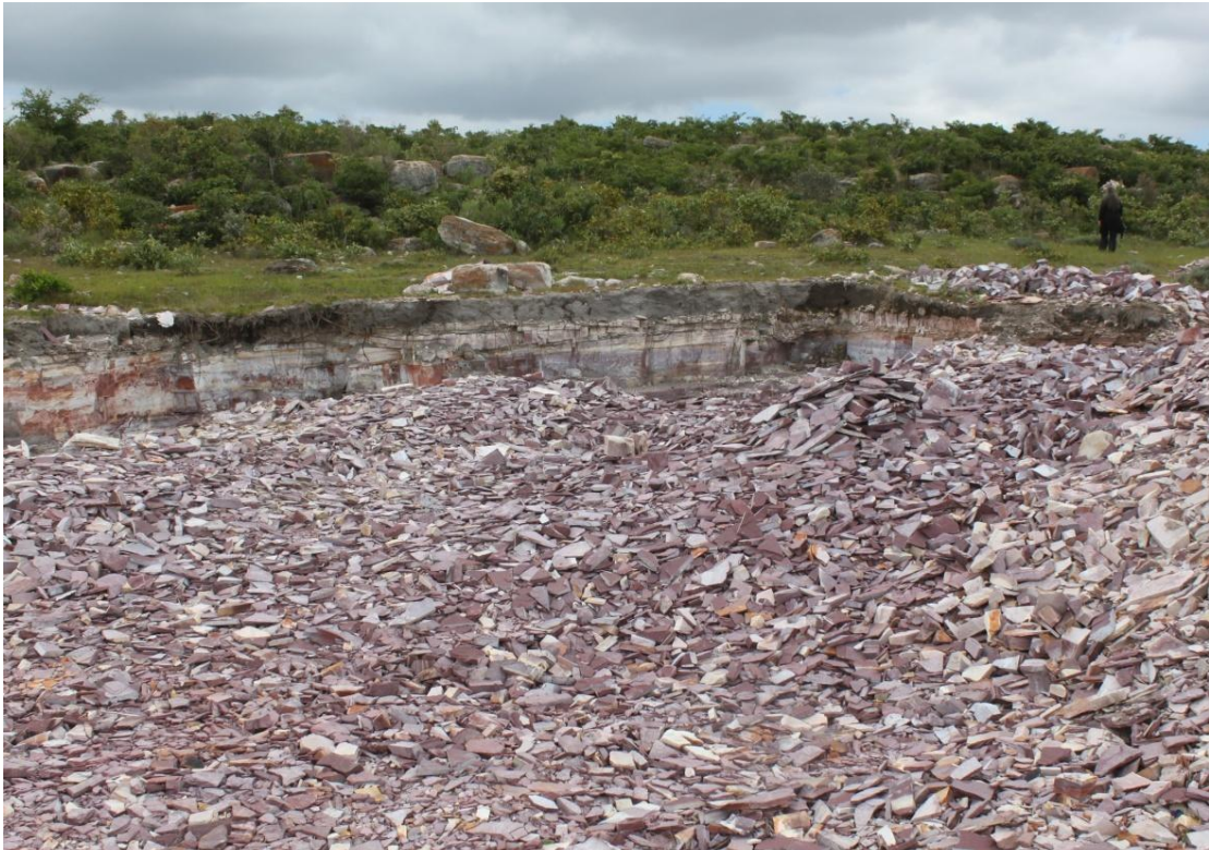
Figure 4.14 – Hand dug quarry stone (rose quartzite) extraction near “Cristo Rei”
