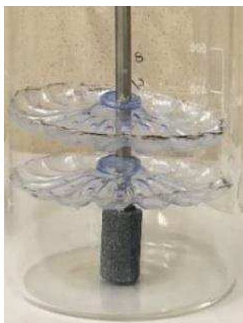
Figure X. 1. Example of biofilter without clams used in the experiments.
