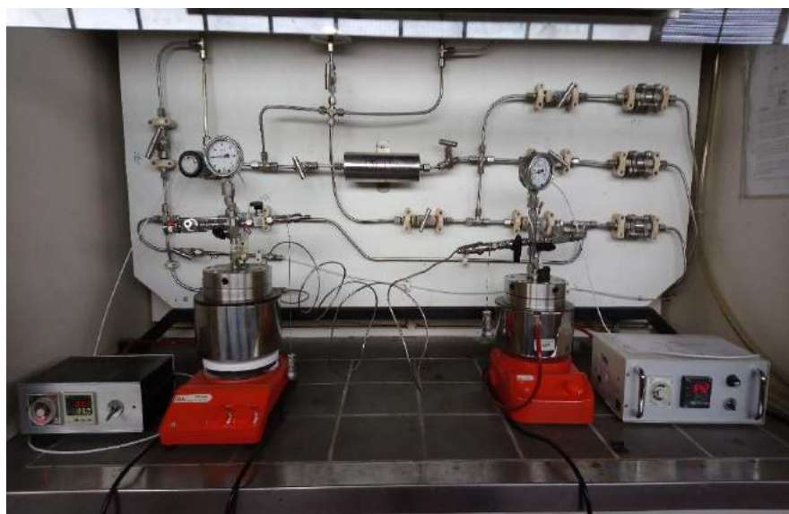
Figure 5.1 – High-pressure system for catalytic sequential epoxidation/ CO_2 cycloaddition (Department of Chemistry, University of Coimbra, Portugal).
