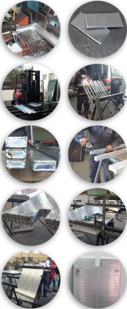
Production of aluminium containers to be used in the TES units
