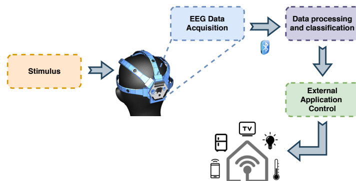
Figure 1.1: Schematic representation of the intended SSVEP-based BCI.
