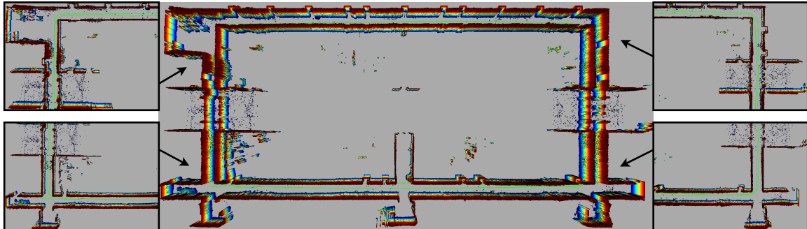
Figure 6.13: Illustration of the 2.5D map generated using 1800 particles in the KLD-based filter for the 2.5D Mapping and Localization approach. The curves have been zoomed for a better visualization
