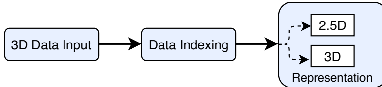
Figure 4.3: Data flow diagram from the point cloud to the desired representation.
