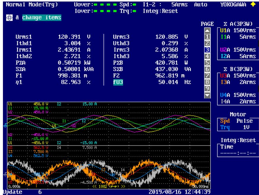
Figure 4.13: Power analyzer results (UPS1) when the linear load is equally shared by the two systems ( $\lambda_1 = 0.5$ ).
