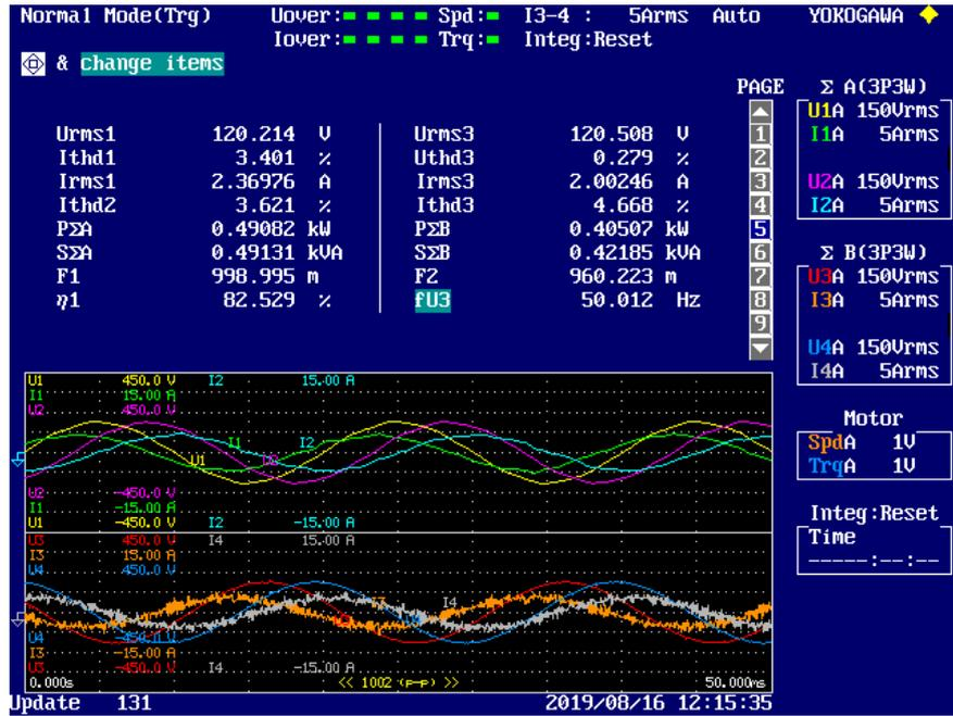
Figure 4.14: Power analyzer results (UPS2) when the linear load is equally shared by the two systems ( $\lambda_1 = 0.5$ ).
