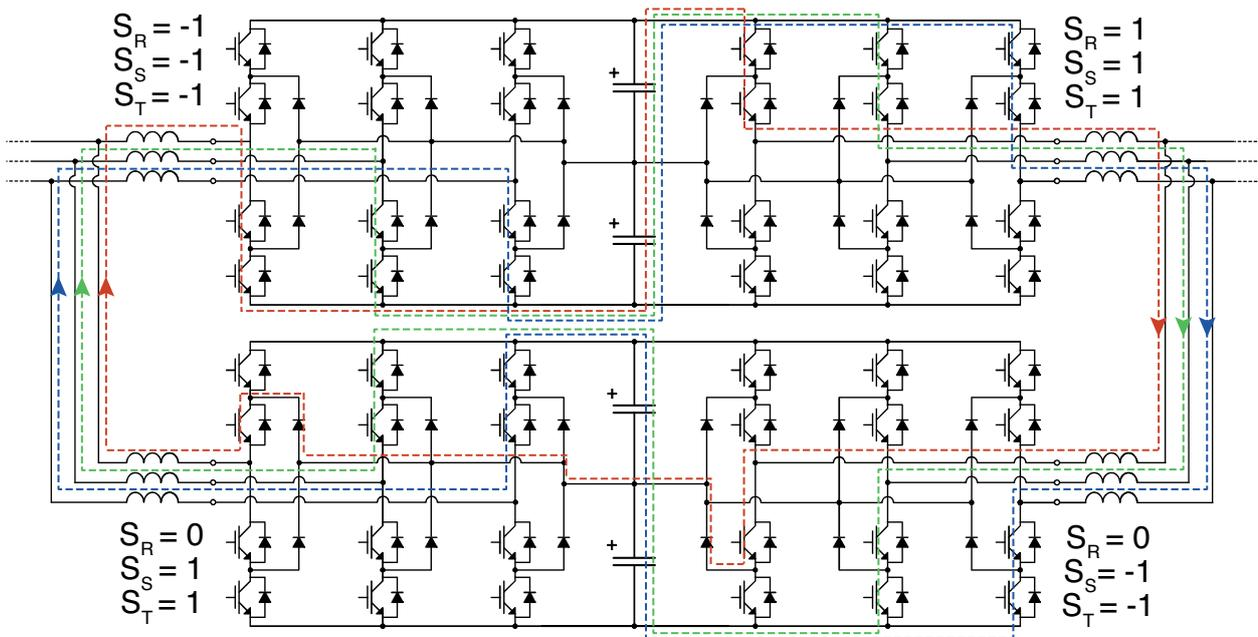
Figure 3.2: Circulating current generation example.
