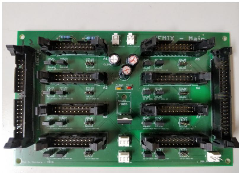
Figure B.14: Pulse directing board (UPS2).
