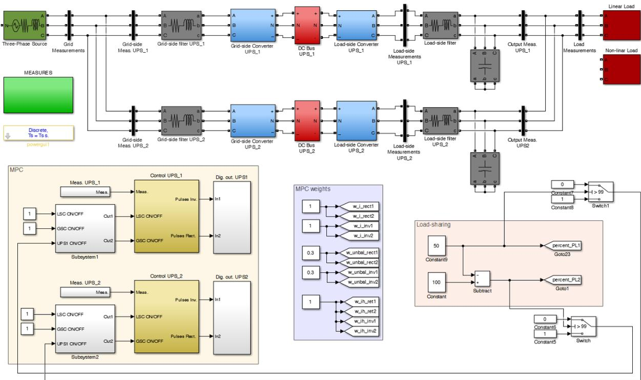
Figure A.1: Overview of the simulation model implemented in *Matlab/Simulink*.
