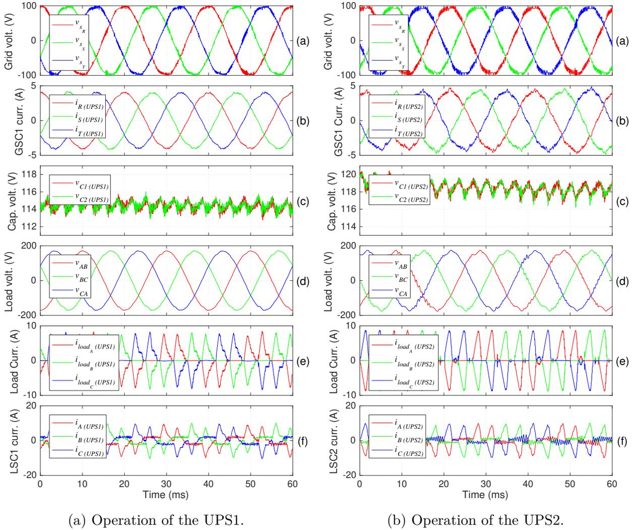
Figure 4.6: Individual UPS performance supplying a non-linear load ( $R=50\ \Omega$ ,  $C=159\ \mu\text{F}$ ) [Experimental].
