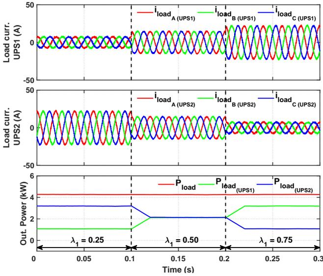
Figure 3. System operation when different percentage of power is assigned to each UPS system ( $W_{i_G} = W_{i_L} = 1, W_{bal_G} = W_{bal_L} = 0.3, W_{z_G} = W_{z_L} = 0.1$ ).
