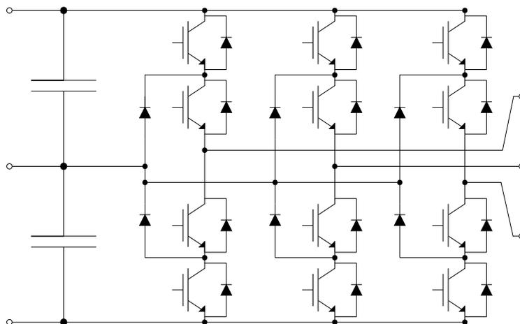
Figure 2.3: Representation of a three-level neutral point clamped (3LNPC) power converter.
