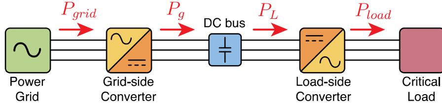
Figure 3.4: Power flow in a single UPS system [2].
