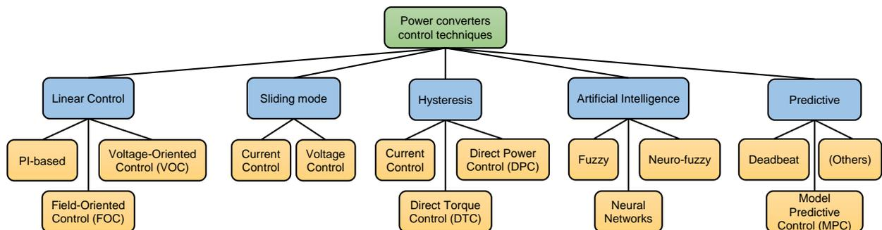
Figure 2.1: Classification of control techniques used for power electronics converters (adapted from [5]).
