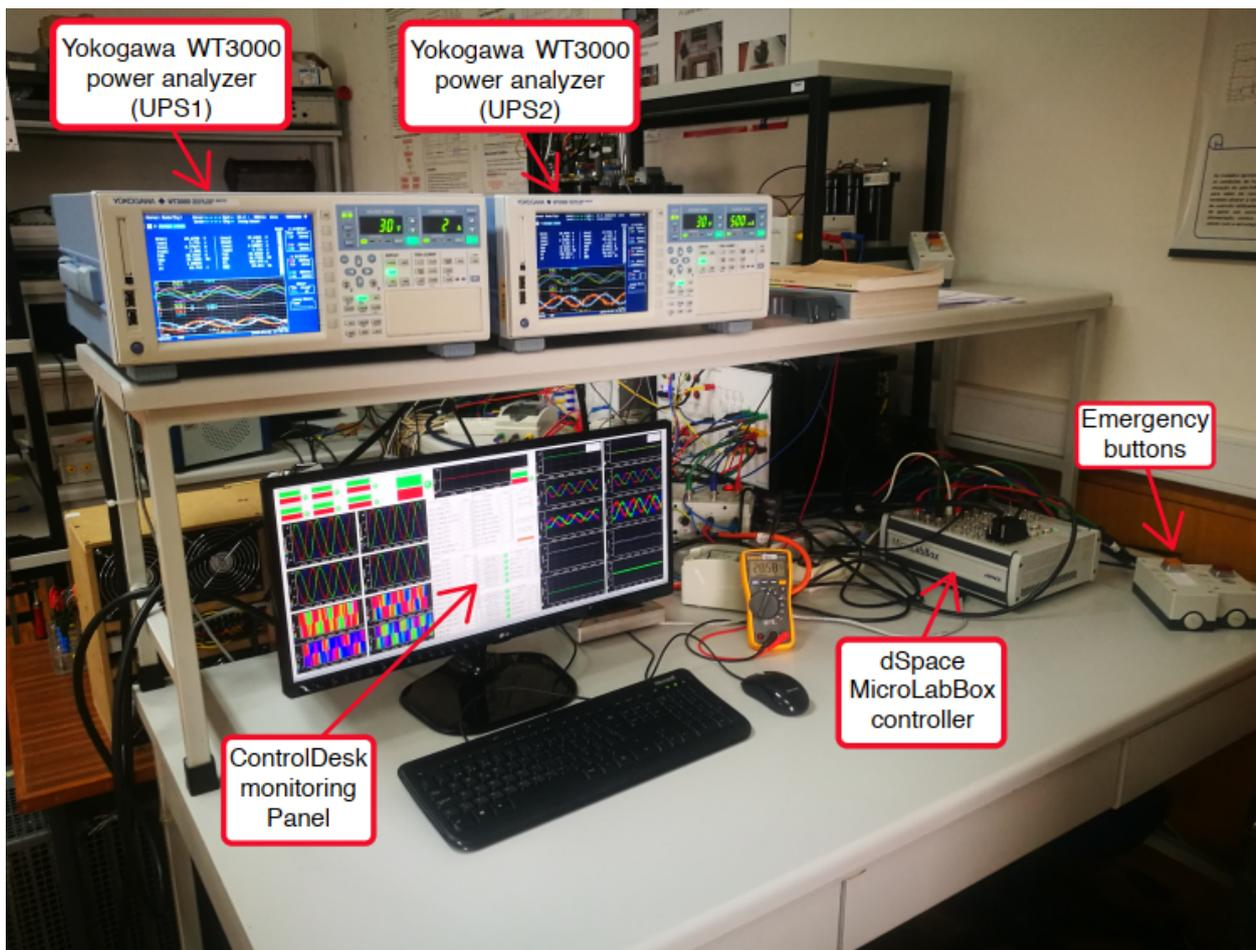
Figure B.2: Global view of the experimental setup and control system.
