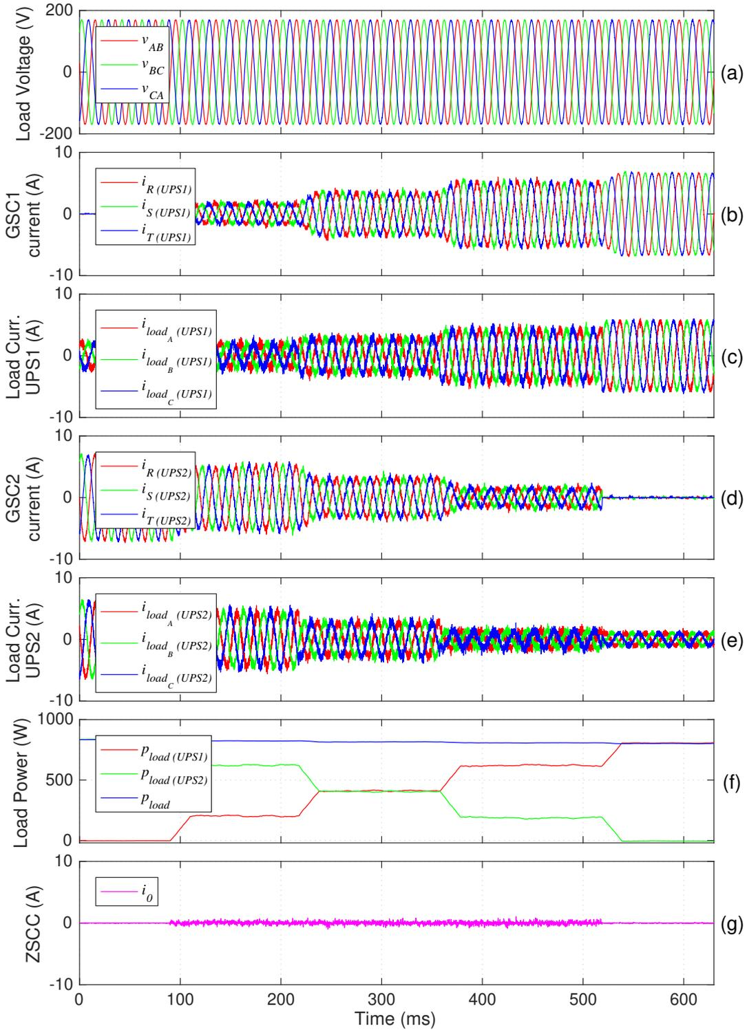
Figure 4.10: UPSs performance when different percentage of the power supplied to a linear load is assigned to each UPS [Experimental].
