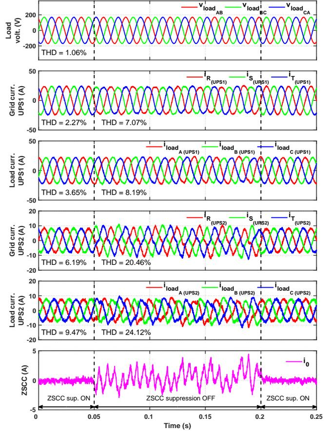
Figure 2. Grid and load currents when system is feeding a linear load w/ UPS1 supplying 75% of load power ( $W_{i_G} = W_{i_L} = 1, W_{bal_G} = W_{bal_L} = 0.3$ ).
