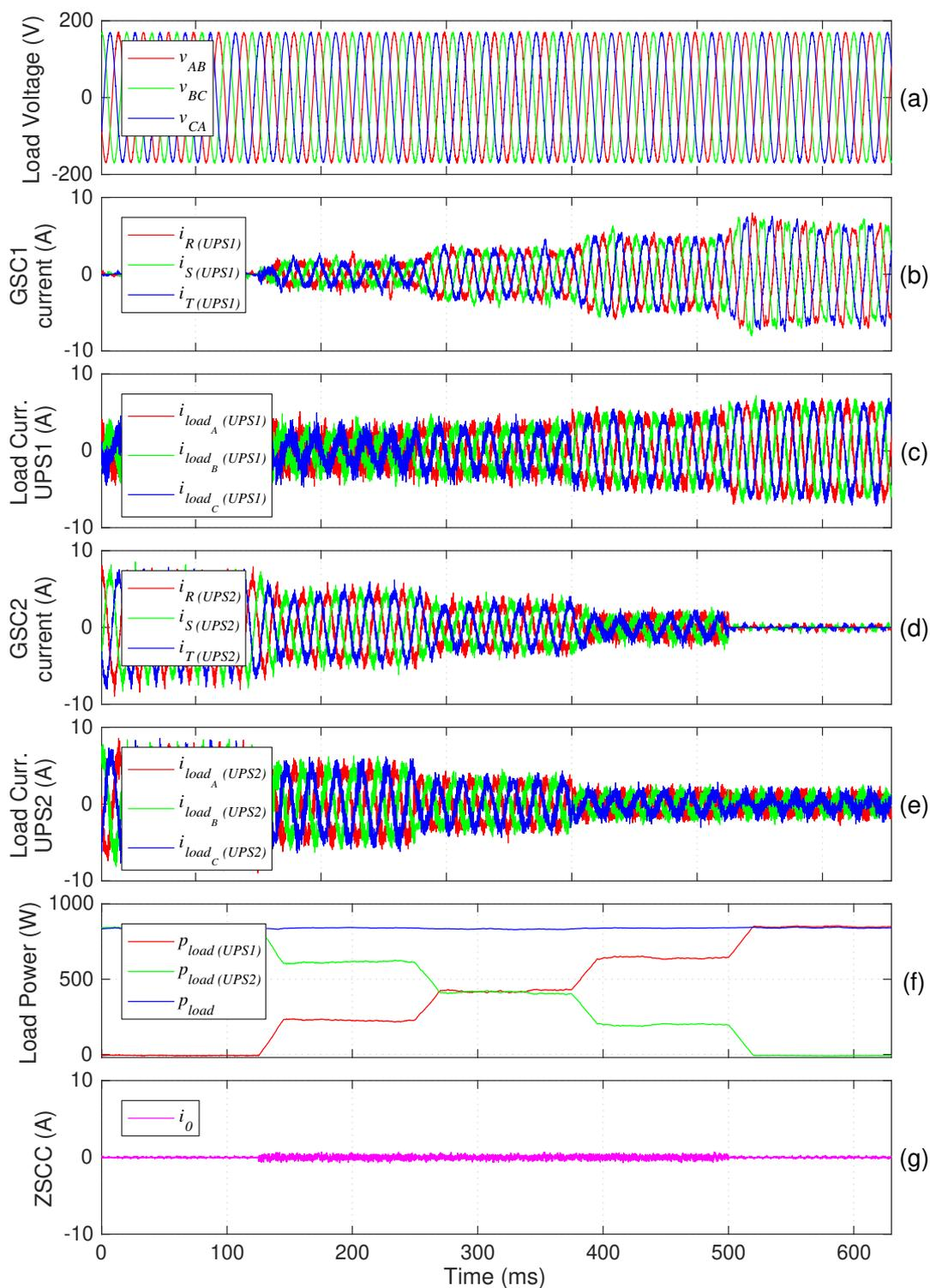
Figure 4.9: UPSs performance when different percentage of the power supplied to a linear load is assigned to each UPS [Simulation].
