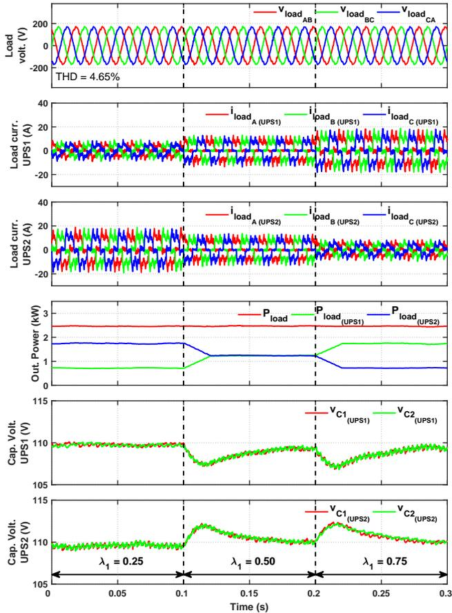
Figure 4. System operation when supplying a highly non-linear load ( $W_{i_G} = W_{i_L} = 1, W_{bal_G} = W_{bal_L} = 0.3, W_{z_G} = W_{z_L} = 0.1$ ).
