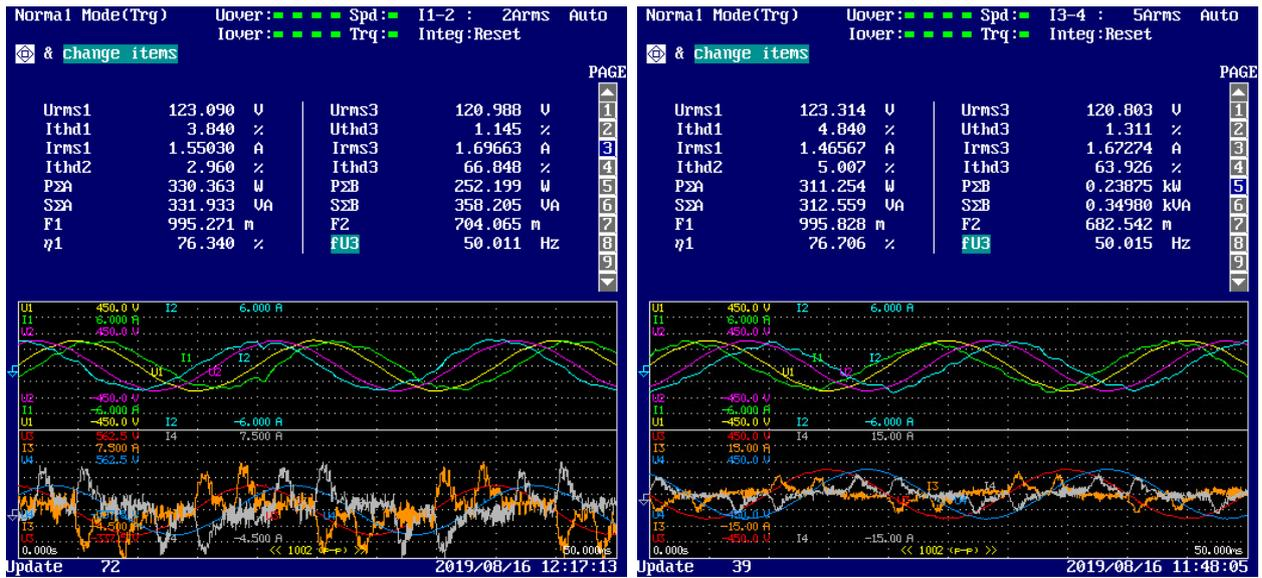
(a) UPS1 providing 50 % of the load power.
