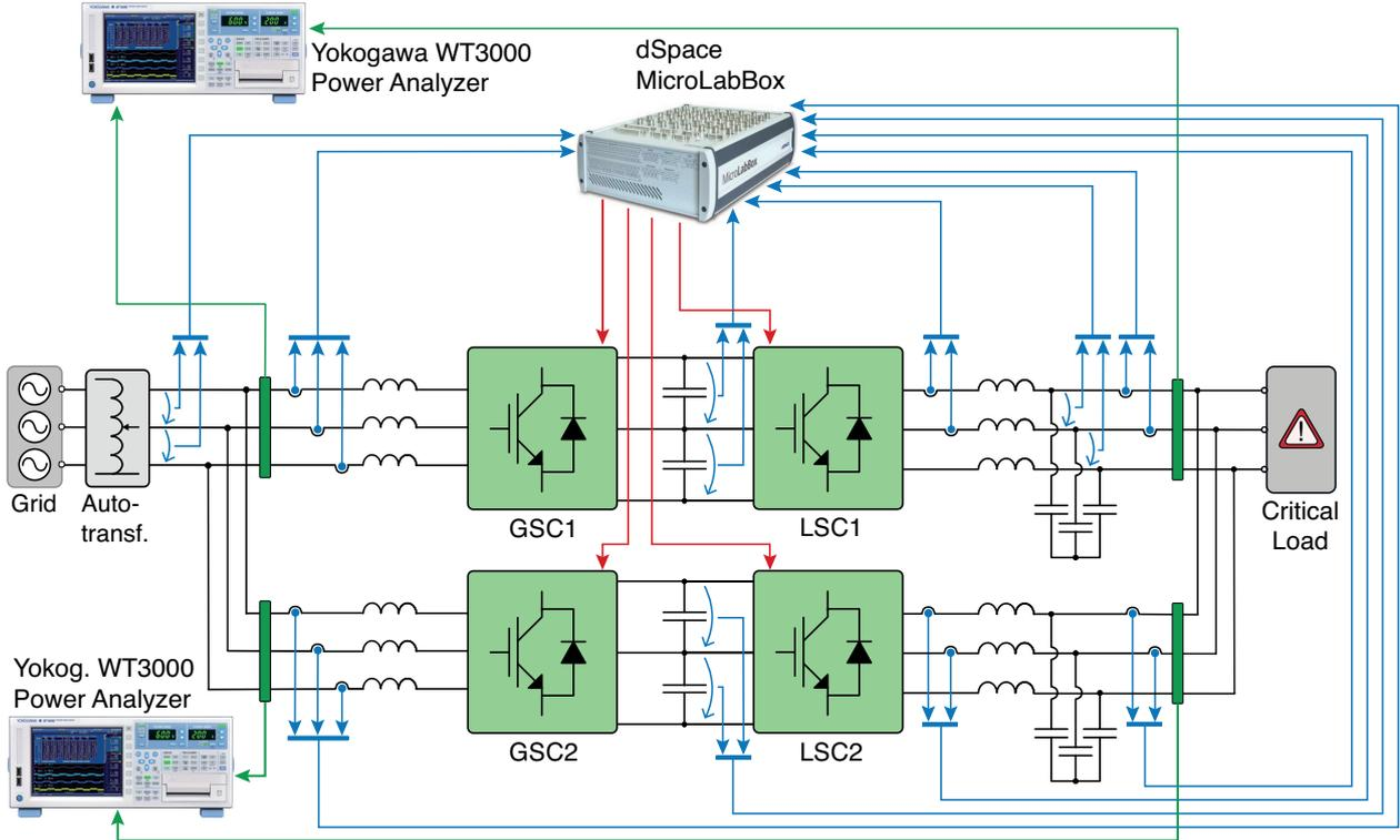
Figure 4.2: Schematic representation of the laboratory setup.
