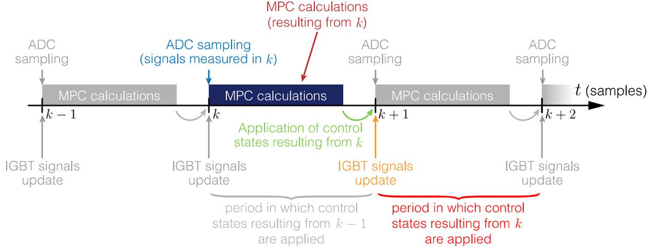
Figure 3.3: Main tasks carried out in a controller during each sampling period (the colored processes are referred to sample  $k$ ) [2].
