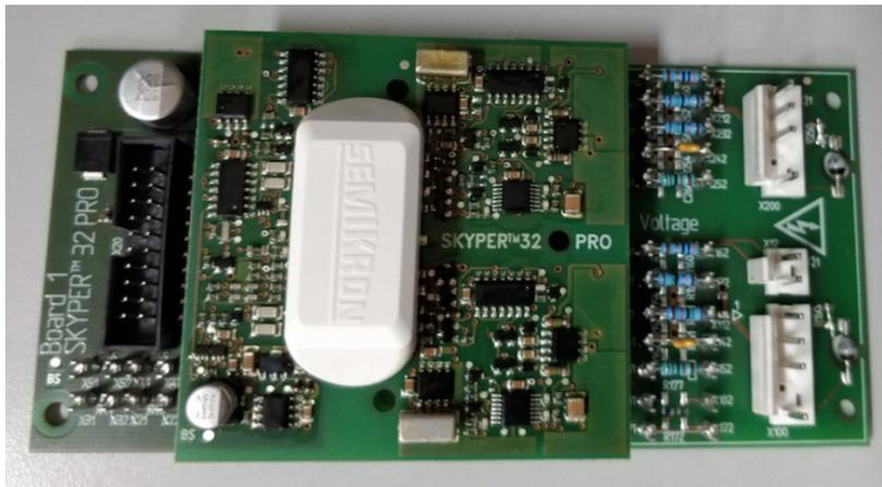
Figure B.12: IGBTs drivers used in UPS2.
