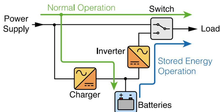
Figure 2.6: Typical configuration of a passive standby UPS [2].
