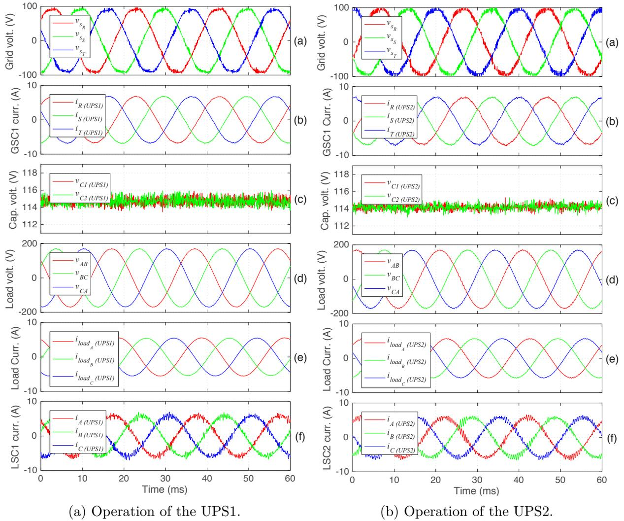
Figure 4.5: Individual UPS performance supplying a linear load ( $R=50 \Omega$ ) [Experimental].
