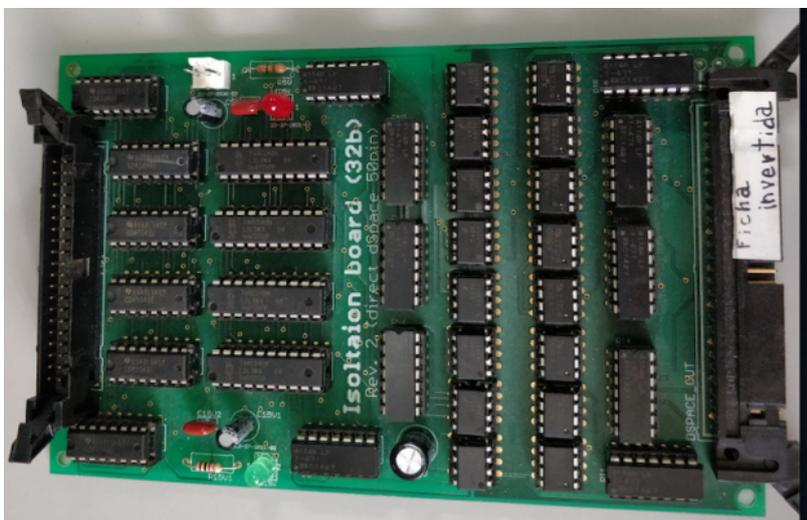
Figure B.13: Isolation board used in UPS2 system.
