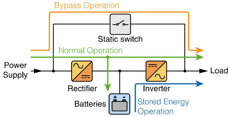
Figure 2.8: Typical configuration of a double-conversion UPS [2].
