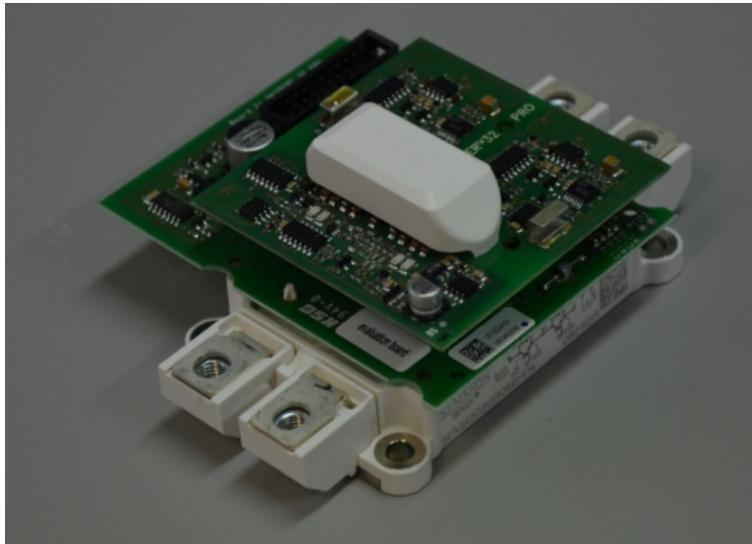
Figure B.8: Half-bridge power modules used in the GSC1 prototype [2].
