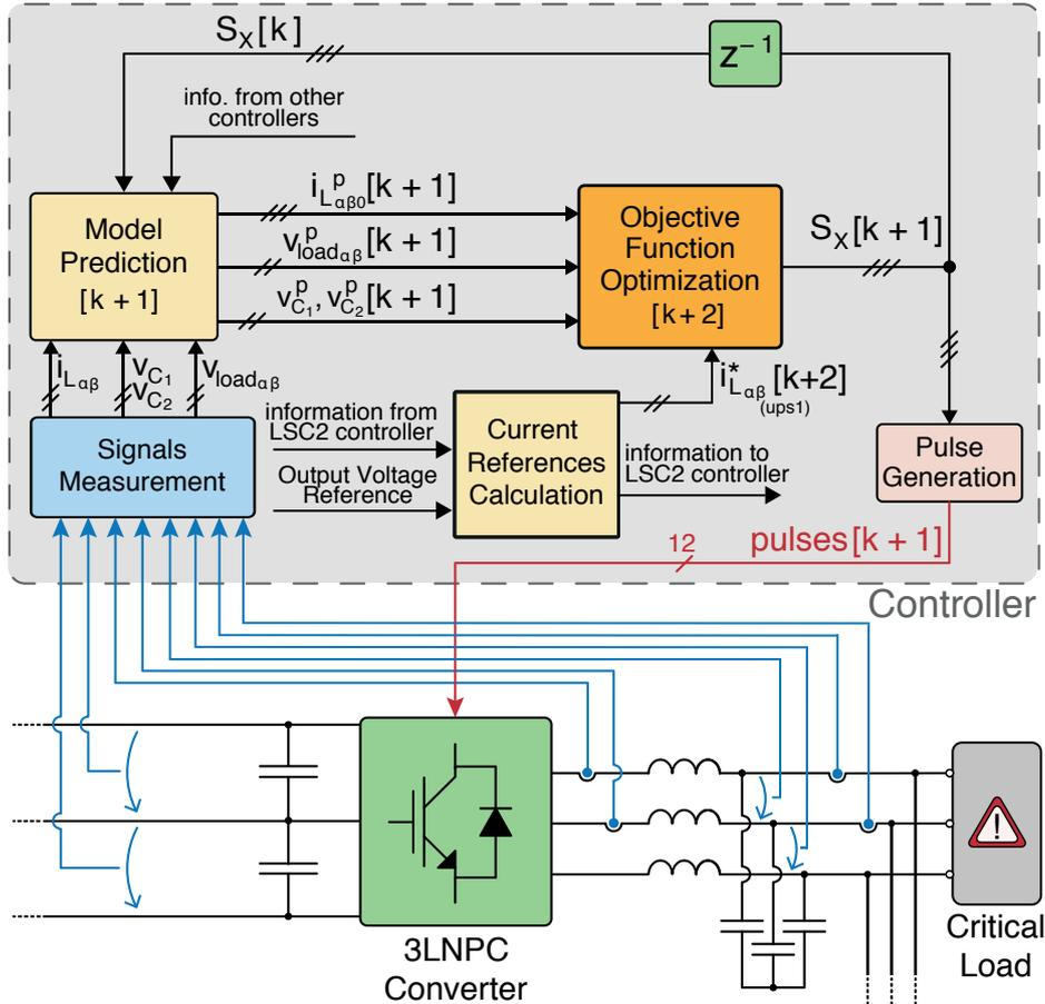
Figure 3.6: Representation of the FCS-MPC strategy implemented to the LSC1 (adapted from [2]).
