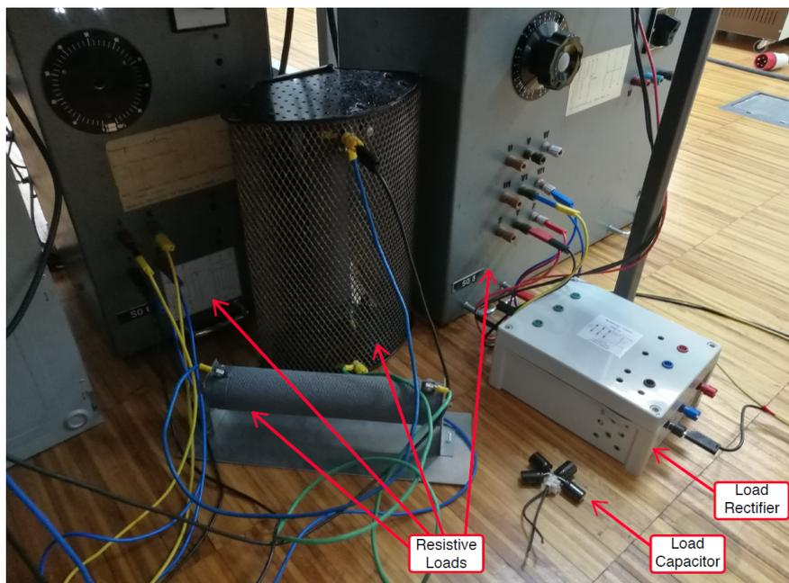
Figure B.20: Loads used in the experimental tests.
