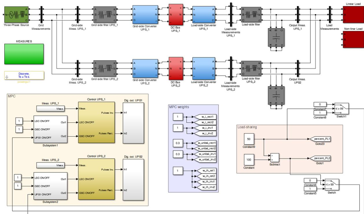
Figure 4.1: Developed simulation model implemented in *Matlab/Simulink*.
