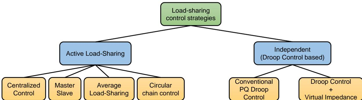
Figure 2.9: Main types of load-sharing control schemes used for paralleled connected UPS (adapted from [31] and [32]).
