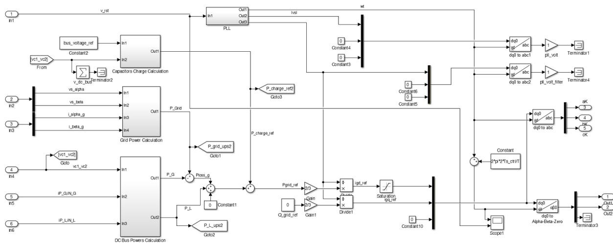
Figure A.4: Overview of the grid current references calculation for the GSC1 implemented in *Matlab/Simulink*.
