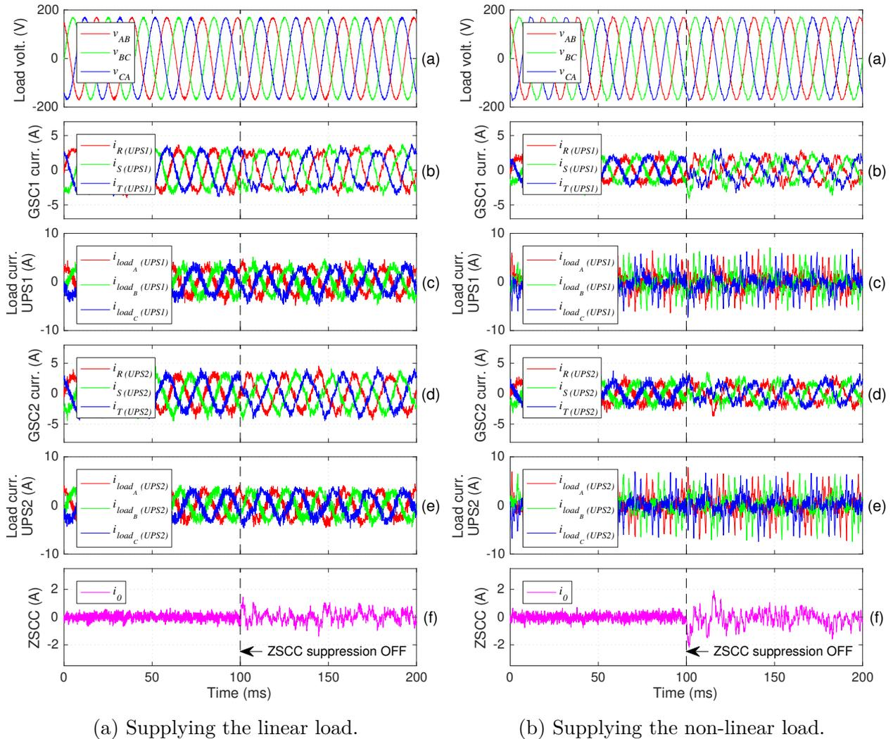
Figure 4.7: UPSs performance during the deactivation of the ZSCC suppression [Simulation].
