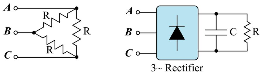
Figure 4.4: Types of critical loads used for the experimental tests.
