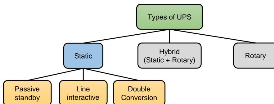
Figure 2.4: Types of uninterruptible power supplies.
