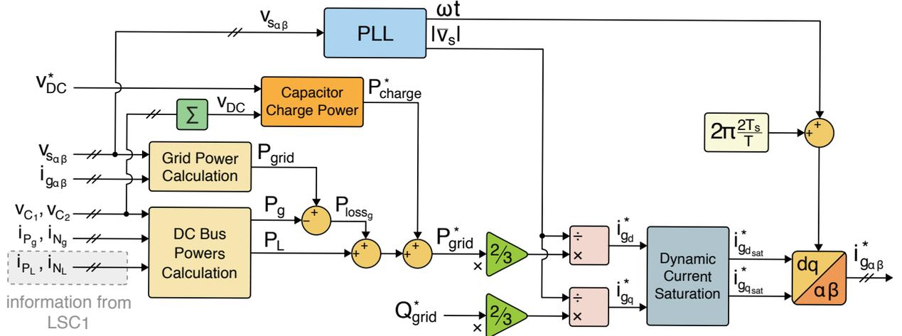
Figure 3.5: Schematic of the GSC1 current references calculation (adapted from [2]).
