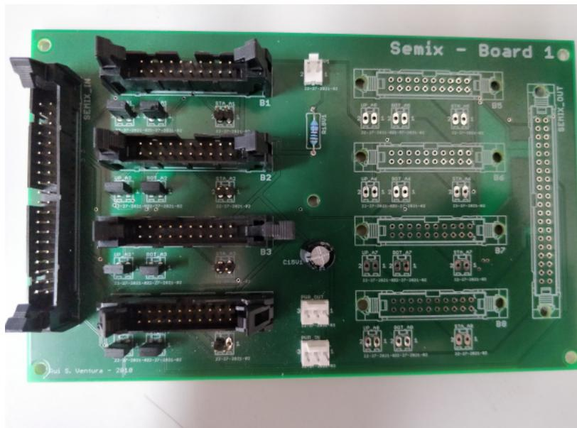
Figure B.15: Pulse directing board (UPS2).
