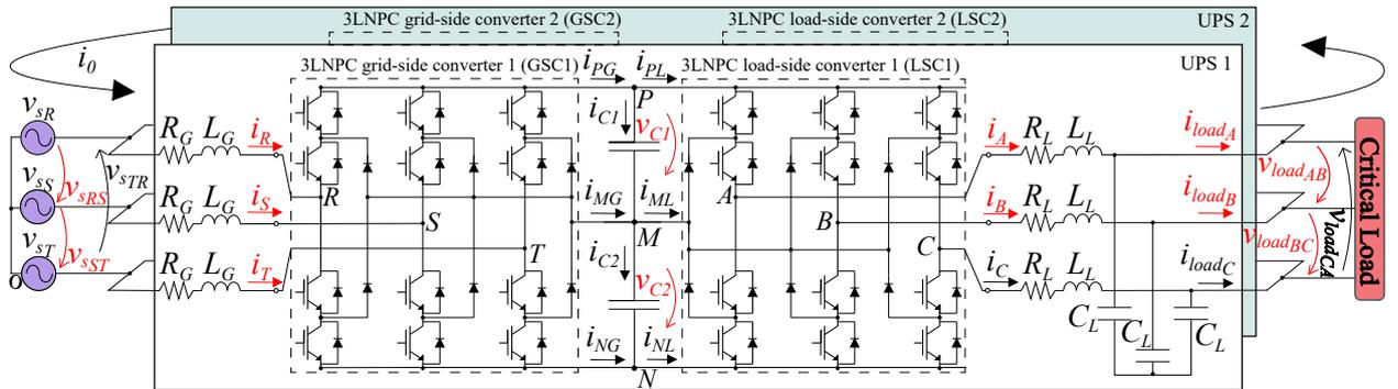
Figure 3.1: Circuit diagram of the proposed paralleled system.
