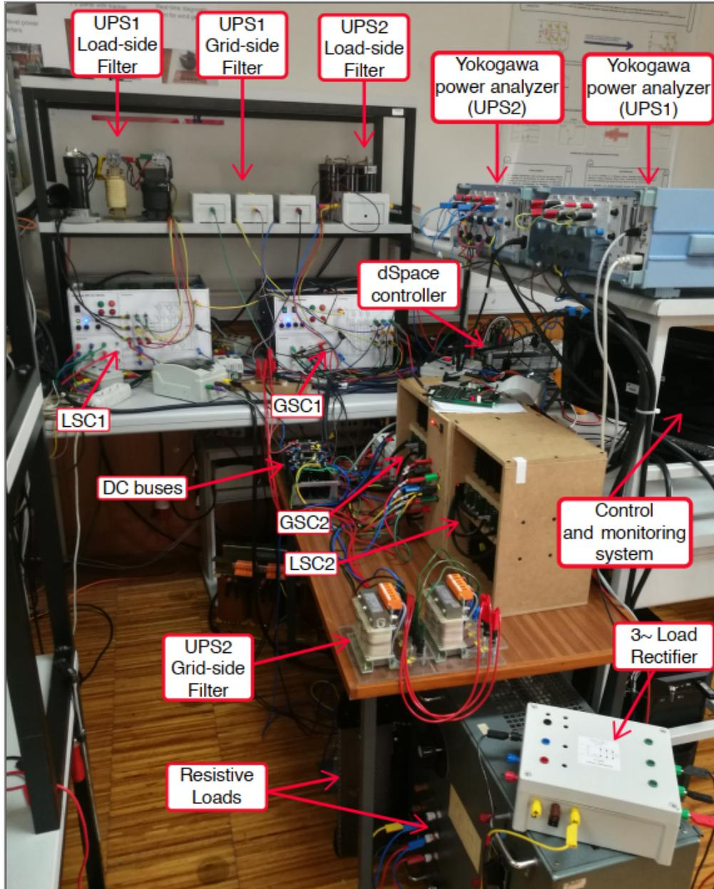
Figure 4.3: Experimental setup of the full system.
