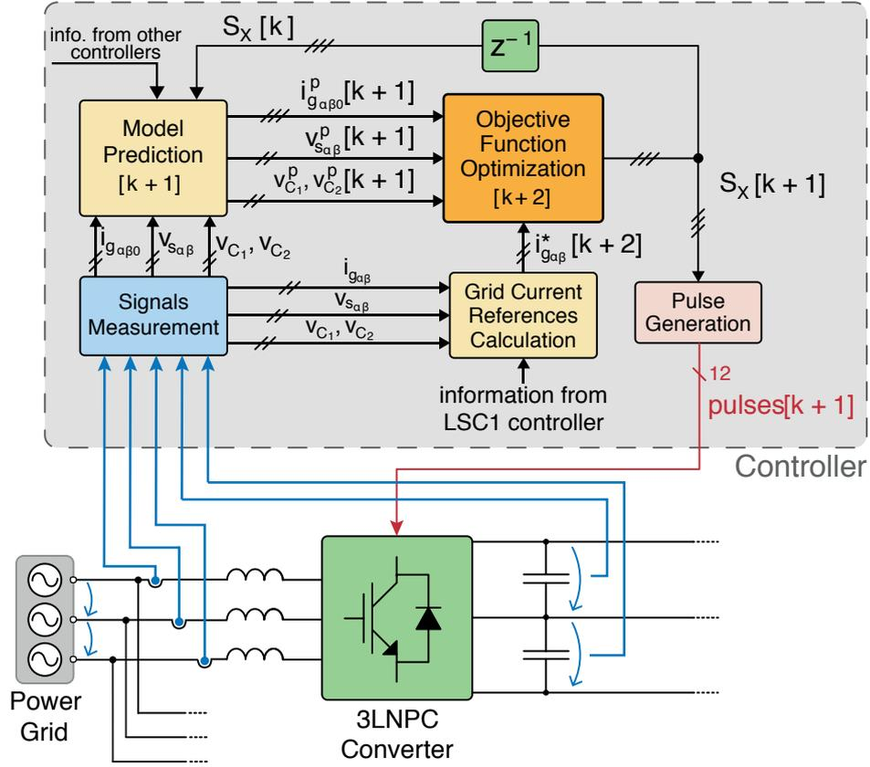
Figure 3.8: Representation of the FCS-MPC strategy implemented to the GSC1 (adapted from [2]).
