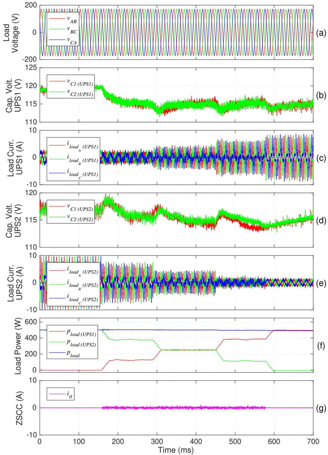
Figure 4.12: UPSs performance when different percentage of the power supplied to a non-linear load is assigned to each UPS [Experimental].
