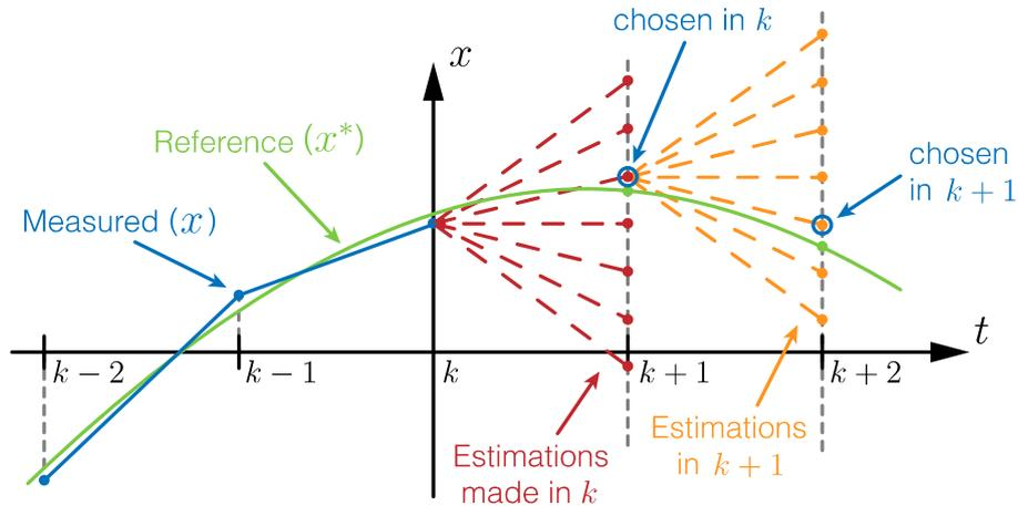
Figure 2.2: FCS-MPC operation principle illustration (adapted from [2]).
