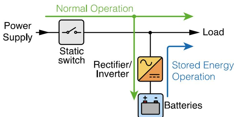
Figure 2.7: Typical configuration of a line-interactive UPS [2].
