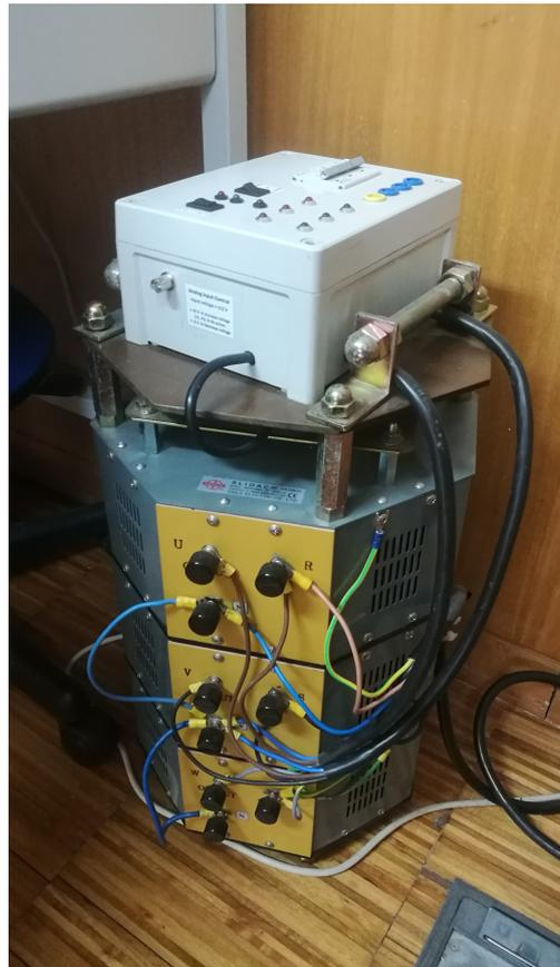
Figure B.19: Autotransformer.
