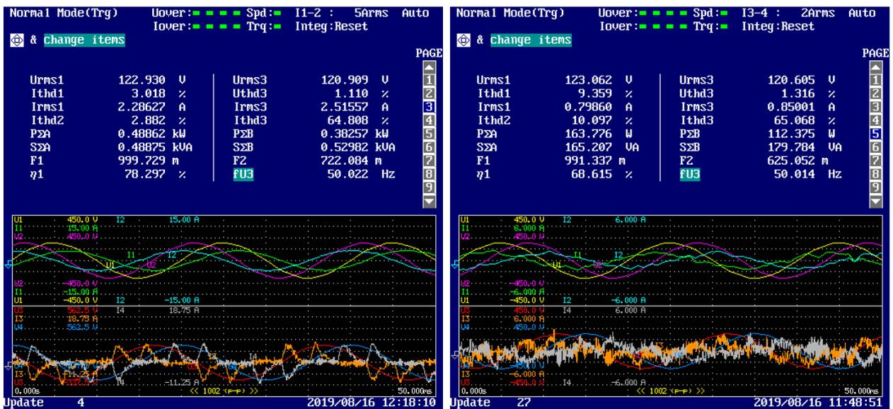
(a) UPS1 providing 75 % of the load power.
