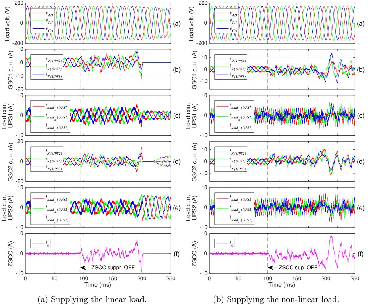
Figure 4.8: UPSs performance during the deactivation of the ZSCC suppression [Experimental].
