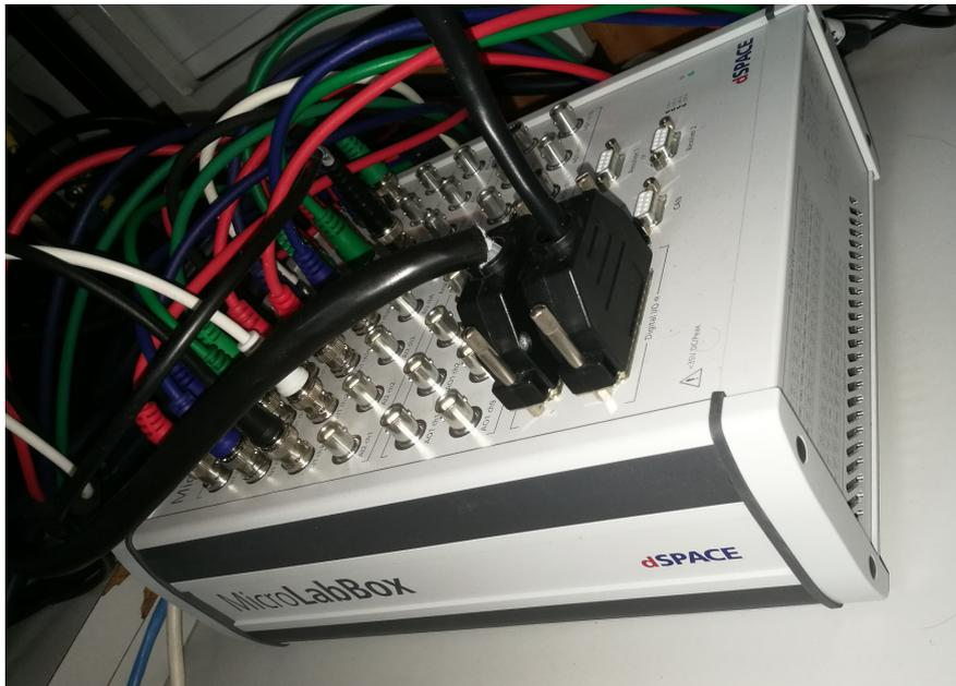
Figure B.17: Used *dSpace MicroLabBox* controller.
