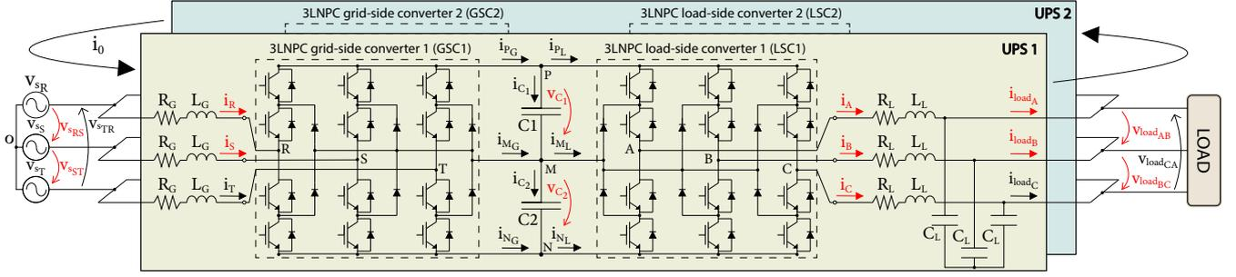
Figure 1. Circuit diagram of the proposed parallel system
