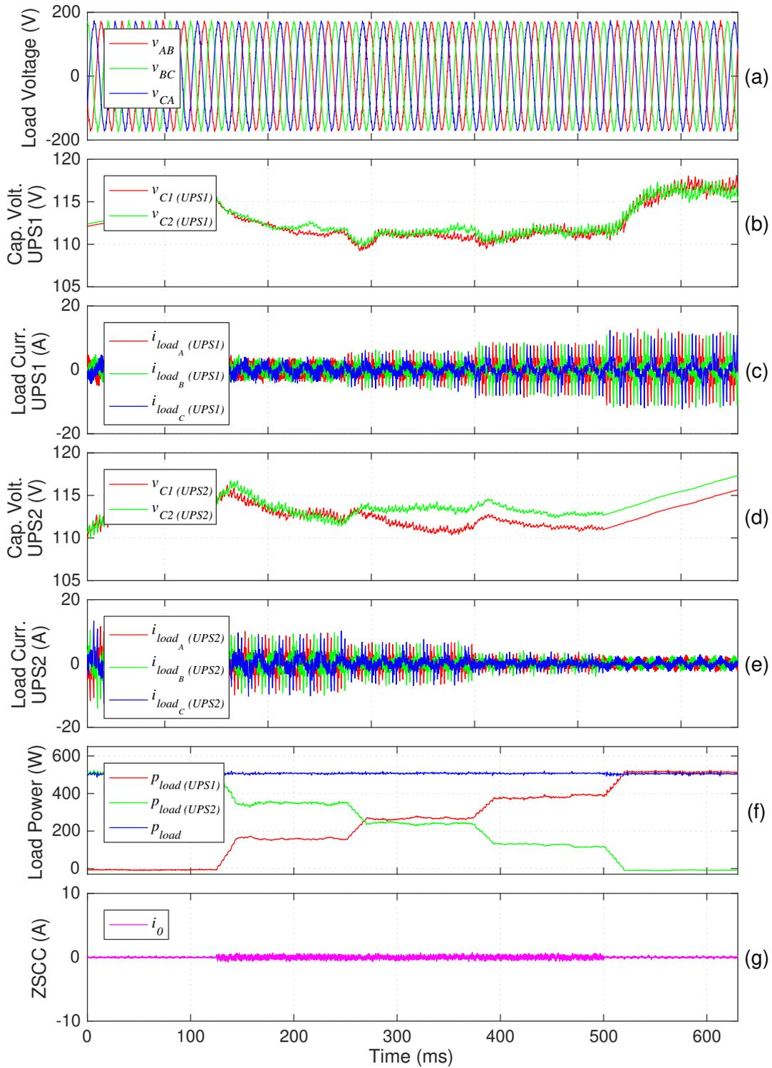
Figure 4.11: UPSs performance when different percentage of the power supplied to a non-linear load is assigned to each UPS [Simulation].
