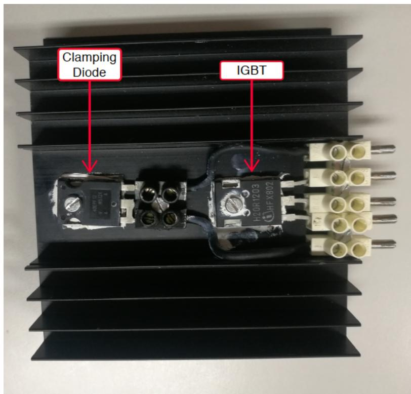
Figure B.11: IGBT and clamping diode (UPS2).
