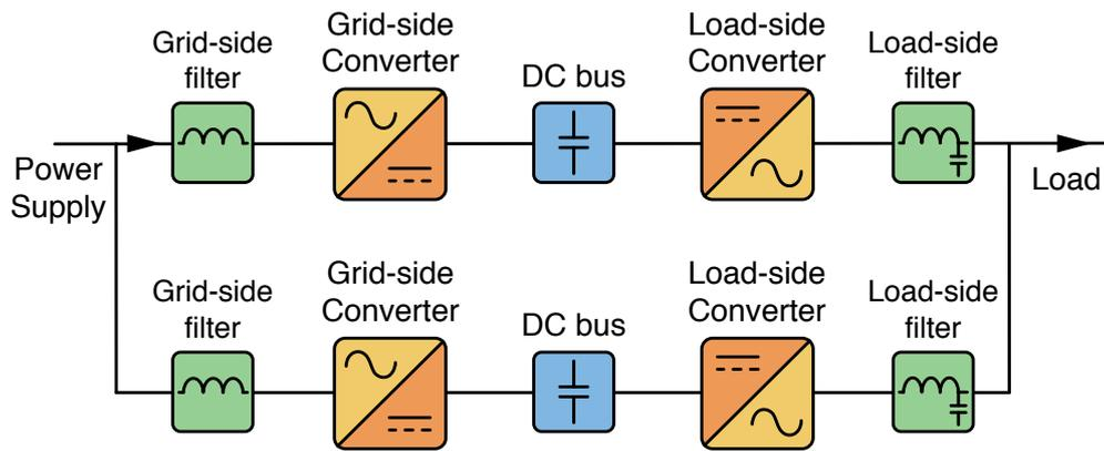
Figure 2.10: Adopted parallel connected system configuration.
