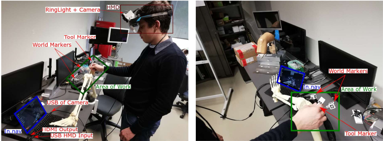
Figure 3.1: Surgical guidance running on an HMD for performing the TKA procedure
