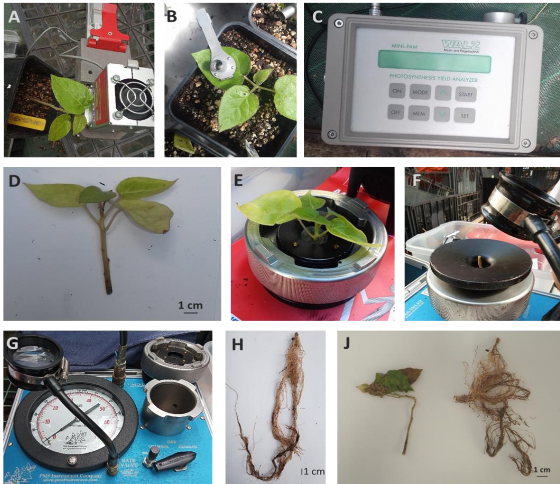
Figure 9 - Plant performance analysis. (A) - Gas exchange parameters assessment; (B and C) – Photosynthetic parameters assessment and portable fluorometer (Mini-PAM; Walz, Effeltrich, Germany), respectively. (D) – Measurement of the plant height; (E, F and G) – Water potential measurement with a Scholander-type pressure chamber (PMS instrument Co., Albany OR. USA); (H) – Plant root after washing; (J) – Dry plant shoot and root for biomass assessment.
