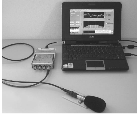
Figure 3 - Sound data-acquisition system – microphone, pre-amplifier, AD board and laptop.
