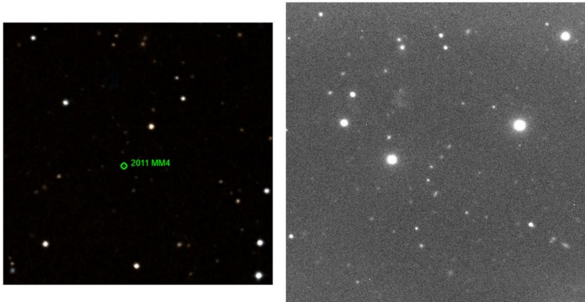
Figure 3.4: 2011 MM4 from AstFinder (left) with the corresponding view from the observation data (right). In this case, the images have similar orientations, but are horizontally inverted.
