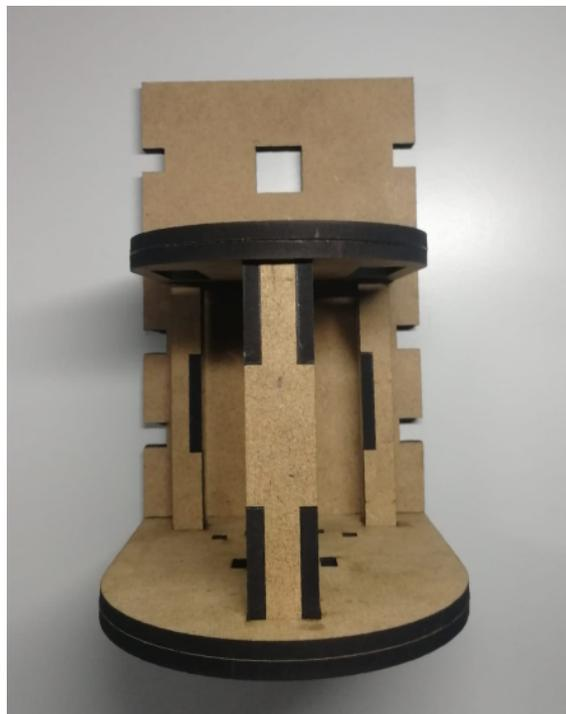
Figure 5.7: Photo of the main piece of the interface assembled without the electronic equipment.
