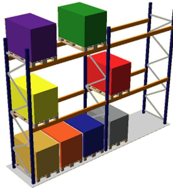
**Figura 4.** Exemplo de *pallet rack: selective rack* (adaptado de Bartholdi, 2011 e Department of the Navy, 1985)
