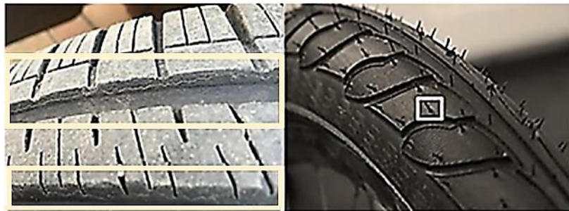
Figure 2.2. Tire molding defects due to: (left side) mold release; (right side) mold fouling – adapted from [13, 14].
