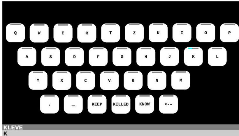
Figure 2.1: Interface of the QWERTZ speller. The n-gram based word suggestions were provided in the lowest row. Source: [25]
