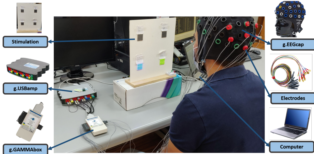
Figure 4.8: Picture of the experimental setup with a user wearing the EEG cap and the g.USBamp amplifier is acquiring the data simultaneous with the occurrence of the stimulation.
