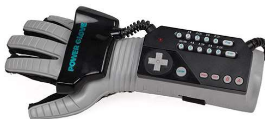
Figura 2.5 – Power Glove controller. 8
