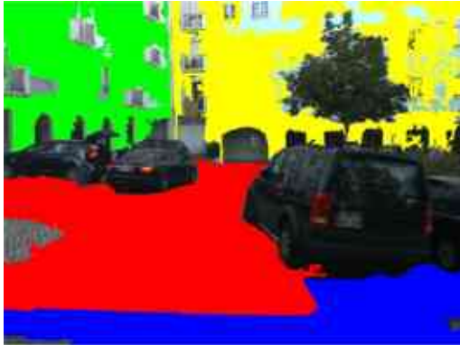
Figure 3.7: Example of a PPR segmentation frame, generated with our algorithm, where we have selected the following combination of planes, for an error measuring: green-yellow, green-red, green-blue, yellow-red, yellow-blue.
