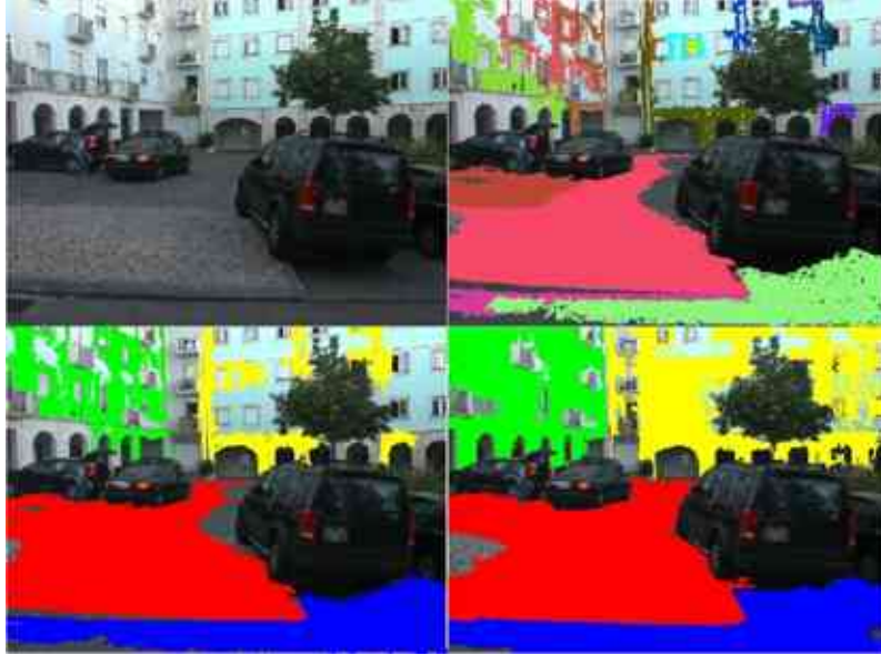
Figure 2.4: Gallup PPR: example illustrating the various stages. First row: (left) Original RGB image, (right) RANSAC plane detection. Second row: (left) Multi-view Plane-Linking, (right) Graph-Cut Image Labeling.
