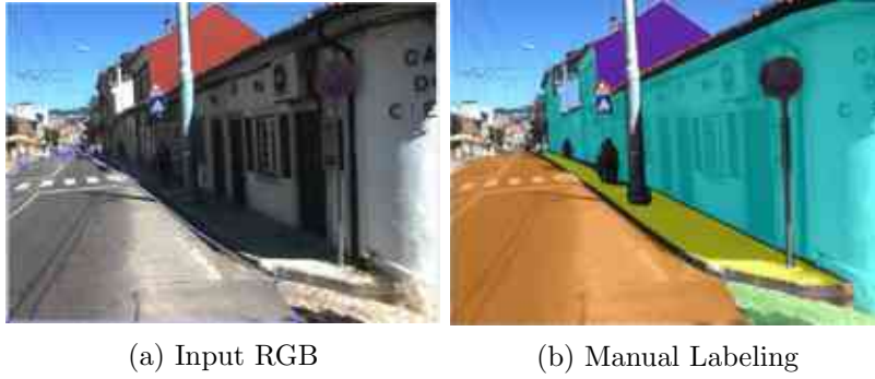
Figure 2.8: Input RGB (left) and the respective fully labelled frame (right), where each color refers to a different plane.
