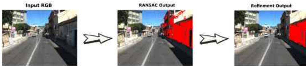
Figure 3.4: Segmentation refinement, after RANSAC returns a plane with the respective inliers. On this example we can observe that some noise was included in the inlier set, which was discarded during the refinement process.
