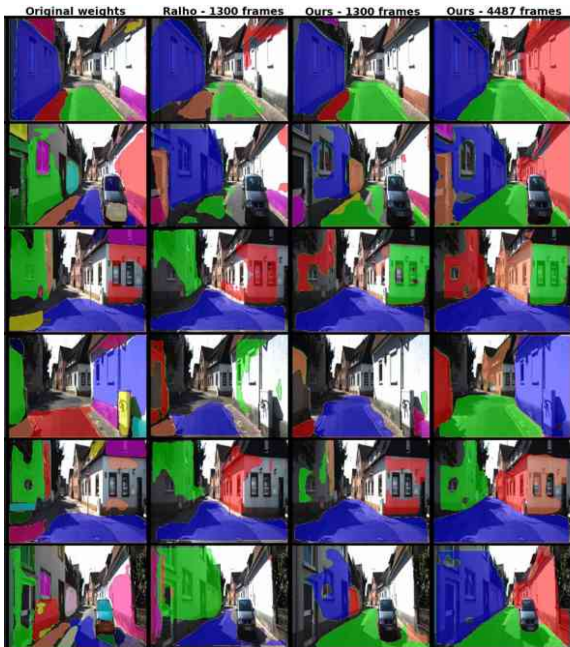
Figure 4.4: Qualitative results for the network output using the Kitti dataset as testset. The figure is divided into three main groups: first and second row contain good and bad results, respectively, obtained with the neural network, after training with all our 4487 frames. Similar to the first two rows, the remaining rows contain good and bad results obtained with the network after training with 1300 PPR segmentation frames from our dataset and Ralho's [1] data, respectively.
