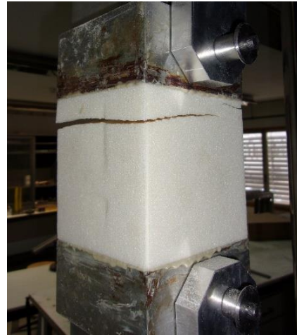
Figure 3-26 - Aspect of PUR board specimen after flatwise tension test.
