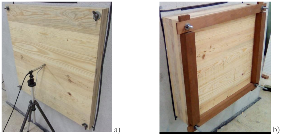
Figure 8-6 - Simplified airborne sound insulation test of: a) CLT 70 panel; b) CIT 170 panel.
