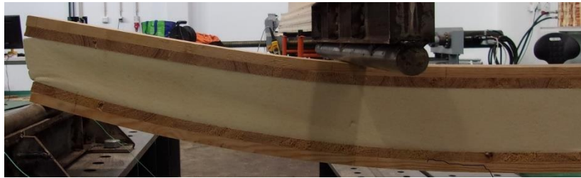
Figure 5-21 – Detail of the deformation of the polyurethane foam during the failure test.
