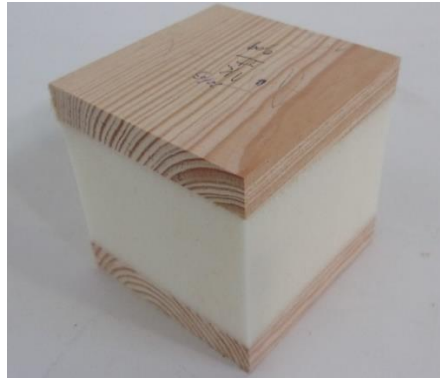
Figure 4-22 – Example of glued polyurethane foam specimen for flatwise tension test.
