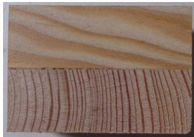
Figure 4-14 – Aspect of glue line' thickness in one of the shear specimens produced with a bonding pressure of 0.1 MPa.
