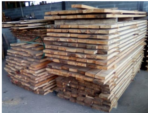
Figure 3-8 – Maritime pine boards classified into strength classes using the timber grader MTG.
