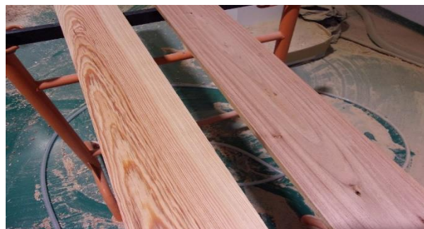
Figure 3-2 – Examples of Maritime pine (left) and Australian blackwood (right) boards after trimming operations.
