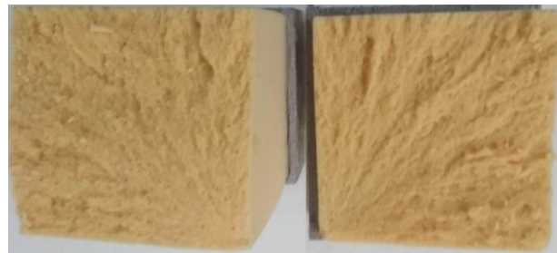
Figure 4-35 – Total failure at the foam observed in a specimen bonded with 1C PUR adhesive subjected to temperature ageing test.
