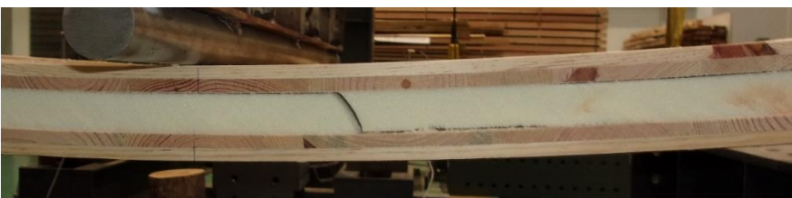
Figure 5-19 - Failure of CIT-10/30-P1
