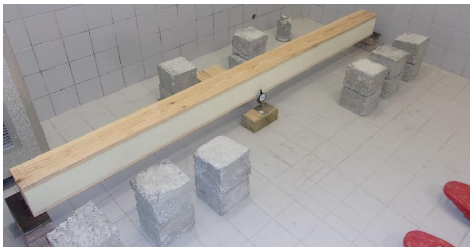
Figure 3-38 – Preparation of the creep test.
