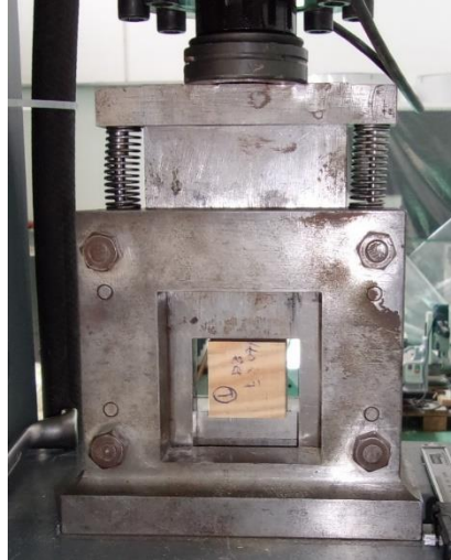
Figure 4-7 – Maritime pine specimen under a shear test.
