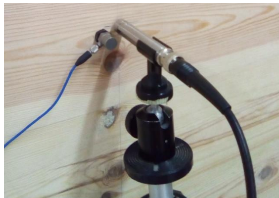
Figure 8-18 – Placement of the microphone and accelerometer.
