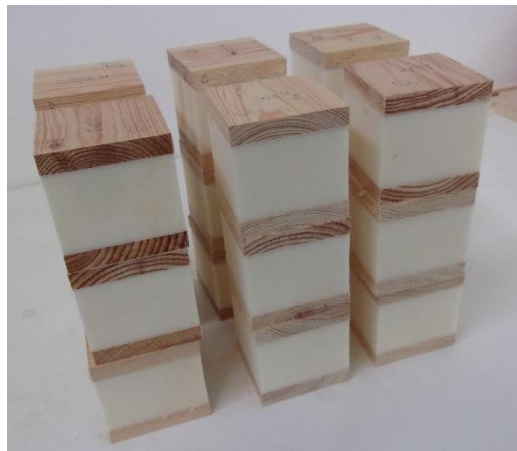
Figure 4-28 – Specimens prepared for the delamination test.
