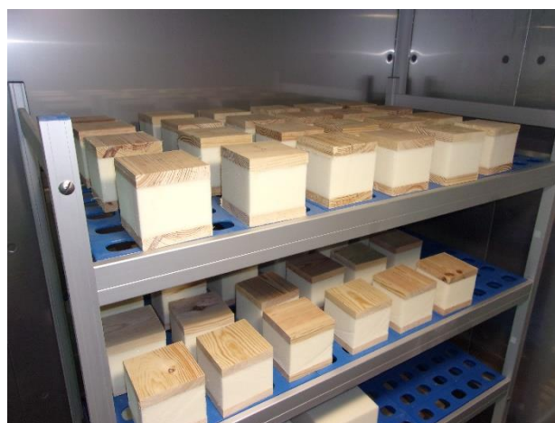
Figure 4-27 – Ageing of the specimens in the climatic chamber.
