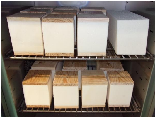
Figure 3-42 – Ageing of specimens in a chamber at 90 °C.
