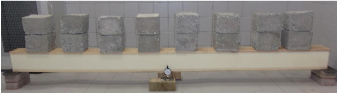
Figure 3-35 - Creep test of a structural insulated panel (SIP) beam.
