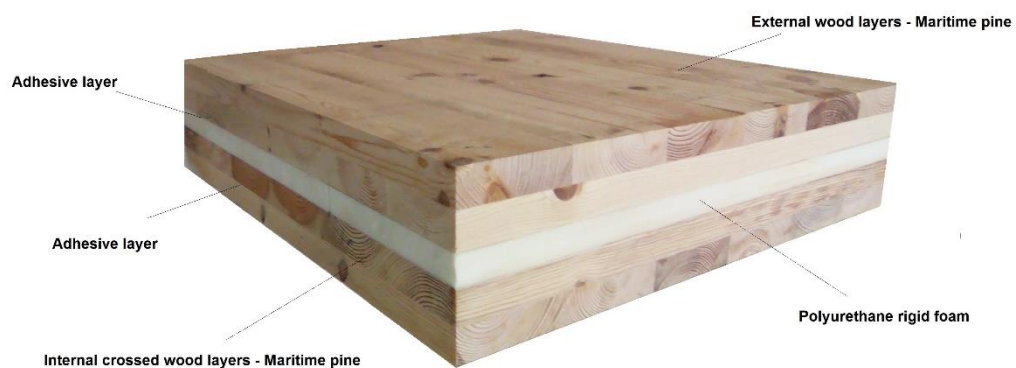
Figure 2-6 – Description of the materials composing the developed panel.
