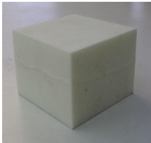
Figure 3-17 - Aspect of a PUR board specimen after a flatwise compression test.
