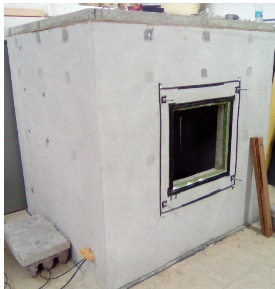
Figure 8-15 – Reduced size-chamber used in the acoustic tests.
