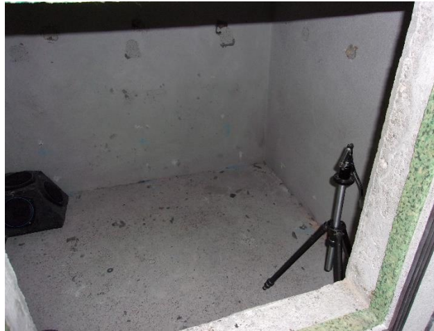
Figure 8-17 – Position of the microphone and sound source inside the chamber.
