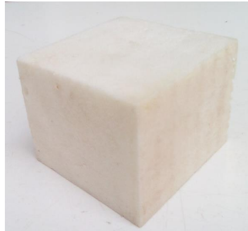
Figure 3-19 - Aspect of an injected PUR specimen after a compression test.
