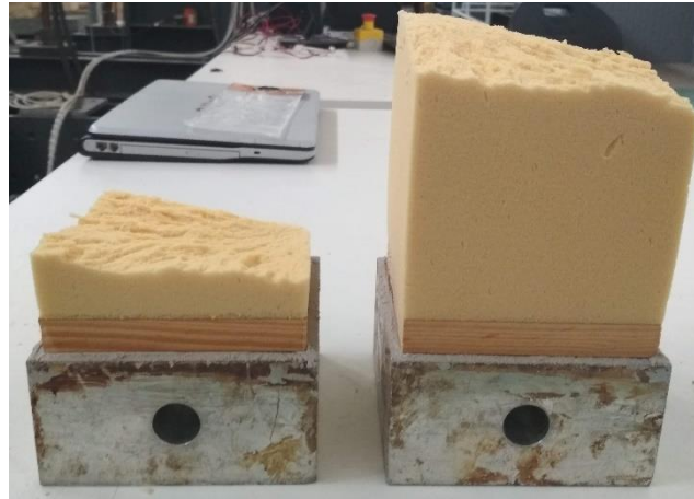
Figure 3-45 – Aspect of PUR board specimen after tension test.
