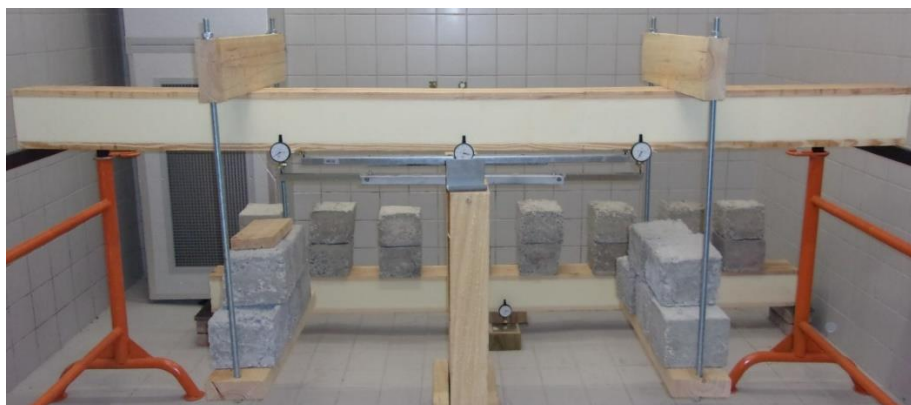
Figure 3-37 – SIP beam tested for measuring the total and local deflection for creep coefficient determination.
