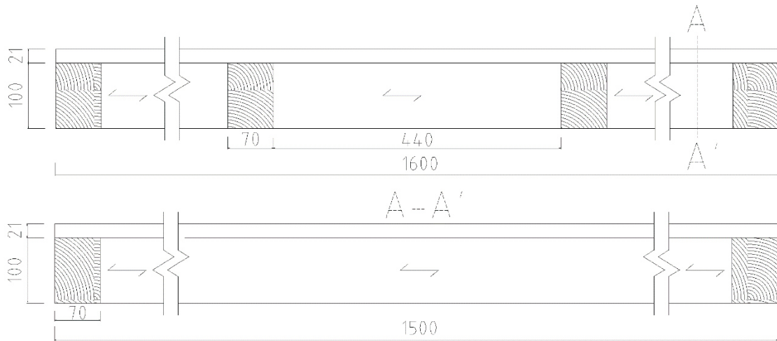
Figure 8-11 – Wood floor dimensions (mm).
