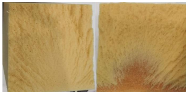
Figure 4-36 – Partial failure at the foam observed in a specimen bonded with 2C PUR adhesive subjected to temperature ageing test.
