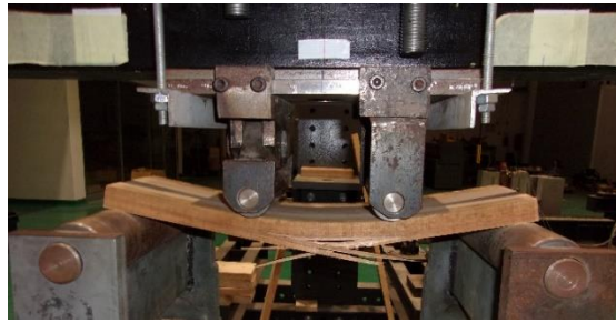
Figure 3-4 – Example of bending test up to failure of an Australian blackwood lamella.
