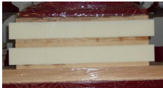
Figure 4-23 – Manufacturing (press) of a beam from which specimens were taken from.
