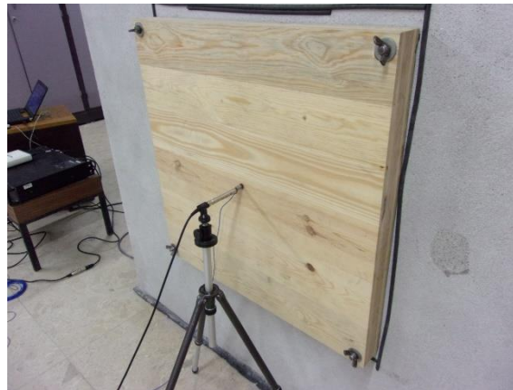
Figure 8-16 – CLT 70 specimen placed on the chamber's opening.
