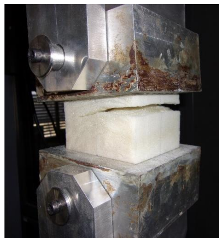
Figure 3-28 - Aspect of injected PUR specimen after tension test.
