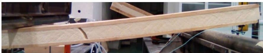
Figure 5-14 – Failure of SIP-10/40-B1.
