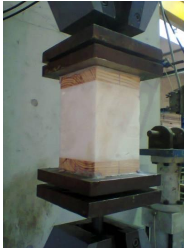
Figure 4-24 – Example of injected polyurethane foam specimen tested in flatwise tension.
