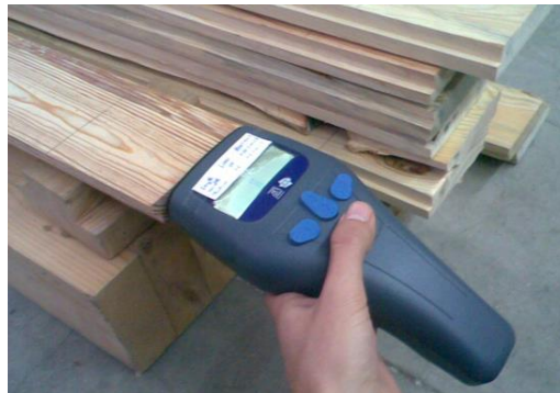
Figure 3-7 – Dynamic test using the timber grader MTG.
