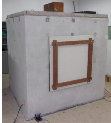
Figure 8-22 – Outside panel for the chamber's closing.
