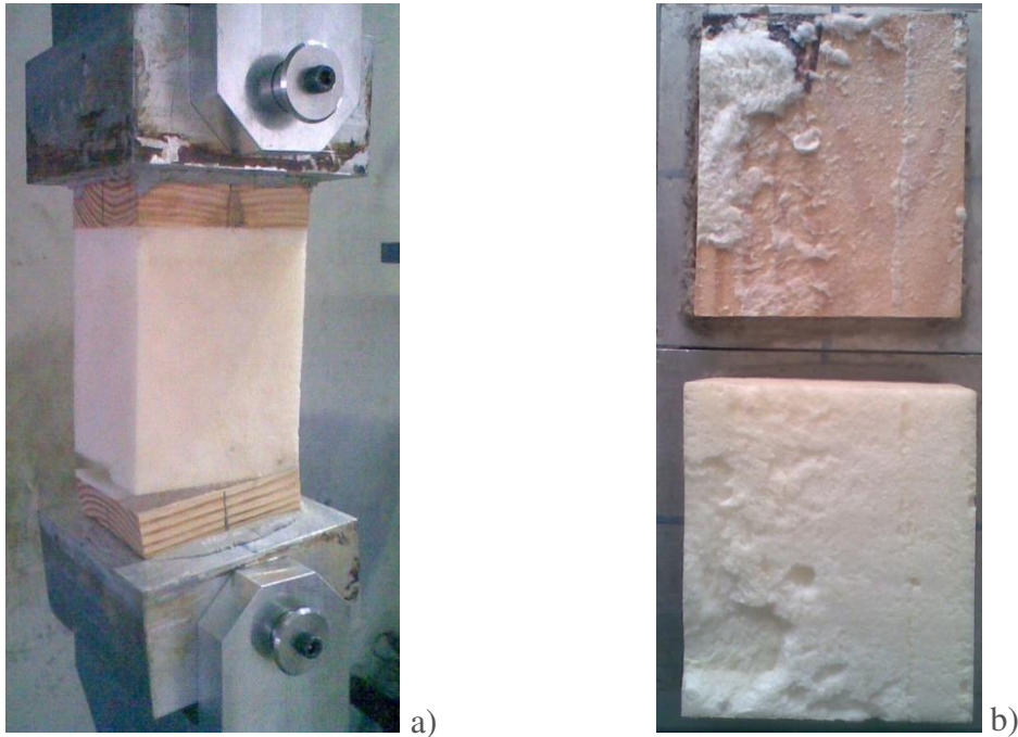
Figure 4-29 - Failure mode in a specimen produced with the injected foam technique: a) delamination at the wood/polyurethane interface; b) aspect of the interface.
