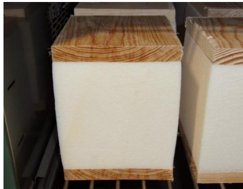
Figure 3-44 – Thickness increase in PUR specimen glued between two wood layers during the ageing test (notice the bending of the foam).
