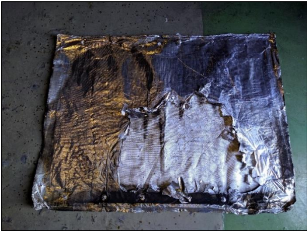
Figure 0.9 - Nozzle CW_02 at a pressure of 3 bar during 2 minutes of exposure.
