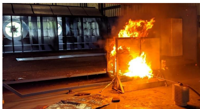
Figure 3.22 - - 2 nd phase tests using nozzle CW_02 and eucalyptus leaves as fuel.
