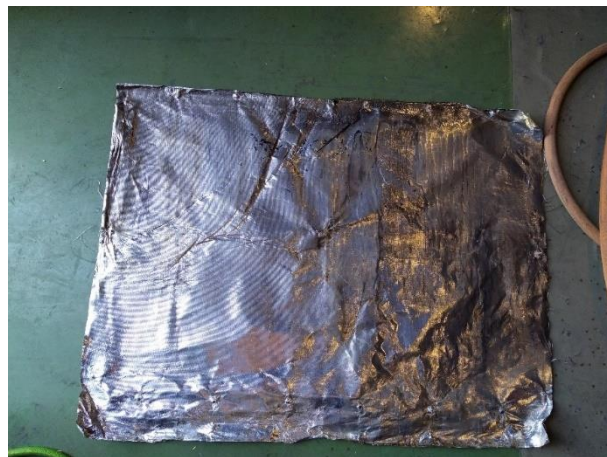
Figure 0.7 - Nozzle CW_02 at a pressure of 2 bar during 2 minutes of exposure.
