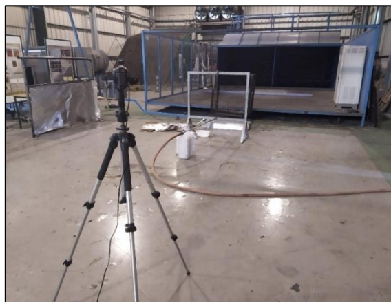
Figure 3.20 – IR camera location in the experiments with fire and airflow tests.
