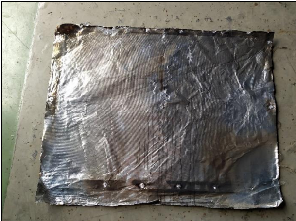
Figure 0.5 - Nozzle AT_02 at a pressure of 3 bar during 2 minutes of exposure.
