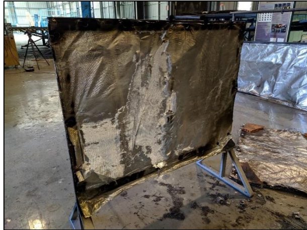
Figure 0.6 - Test without any water system during 2 minutes of exposure.
