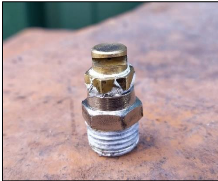
Figure 3.2 - Nozzle CW_01 (spray type).
