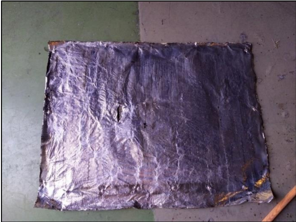
Figure 0.3 - Nozzle CW_02 at a pressure of 3 bar during 2 minutes of exposure.
