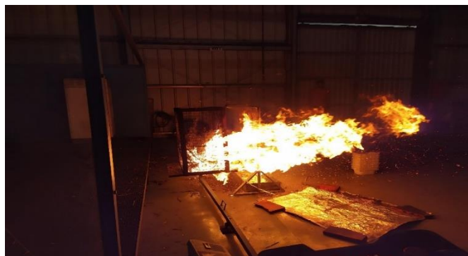
Figure 3.21 – 2 nd phase tests using water spray nozzle type and shrubs as fuel.
