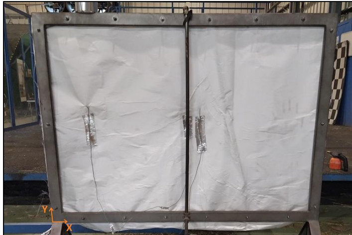
Figure 3.19 – Referential used to locate the thermocouples (back side of the fabric).
