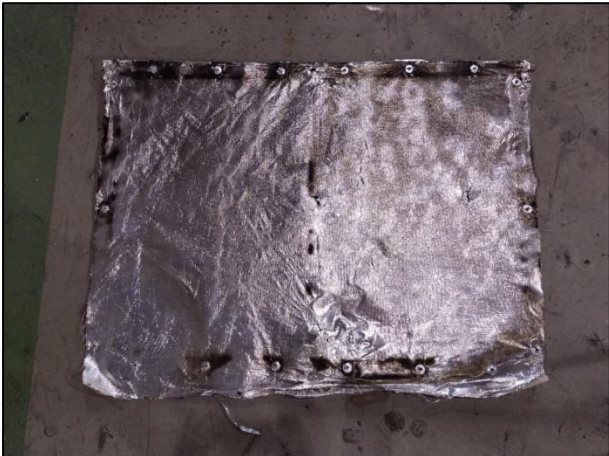
Figure 0.4 - Nozzle AT_01 at a pressure of 3 bar during 2 minutes of exposure.
