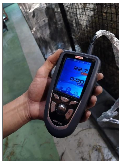
Figure 3.17 – KIMO AMI 300 Hot Wire measurements at the beginning of the tests.
