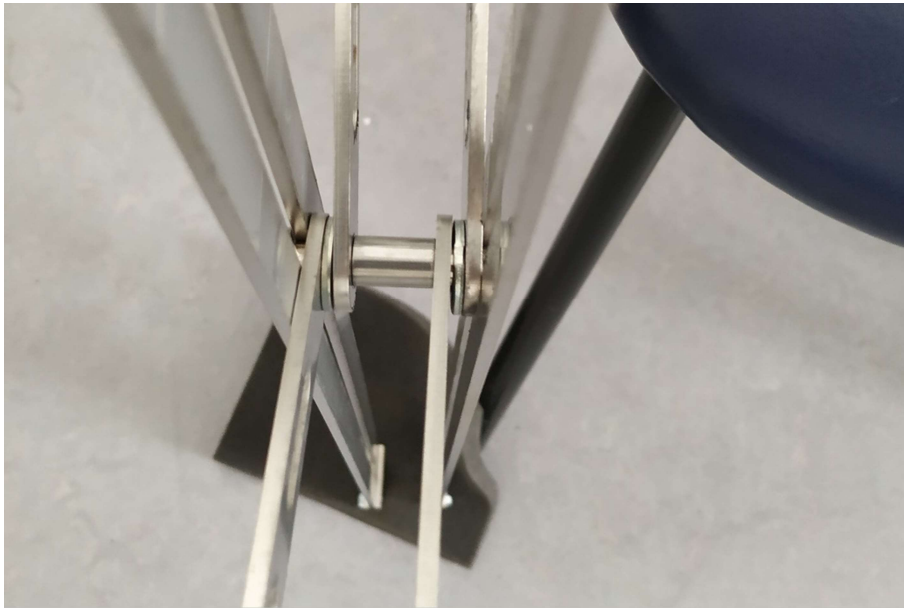
Figure 2.10. Spacer separating the bars.
