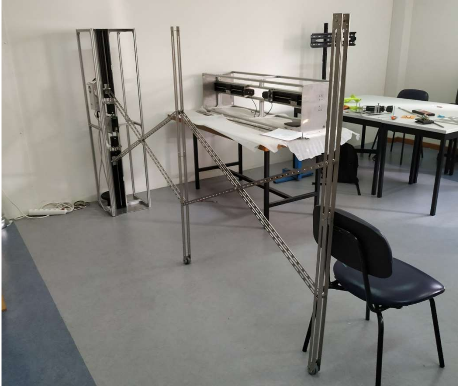
Figure 2.12. First assembly of the structure.
