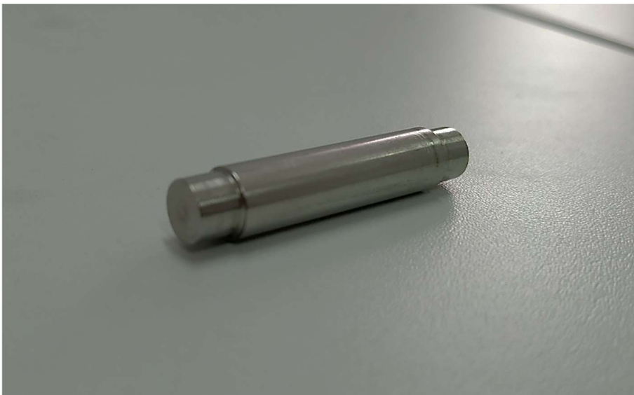
Figure 2.11. Axle for the wheels.
