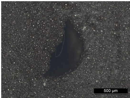
Figure 25 - Vertical insert tips obstructed channel opening detail topography
