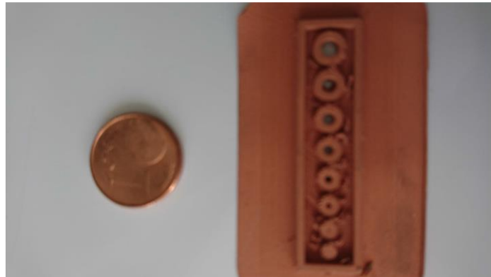
Figure 19 - Prism with several holes aligned, from 0.02 mm to 0.300 mm with an increment of 0.04 mm
