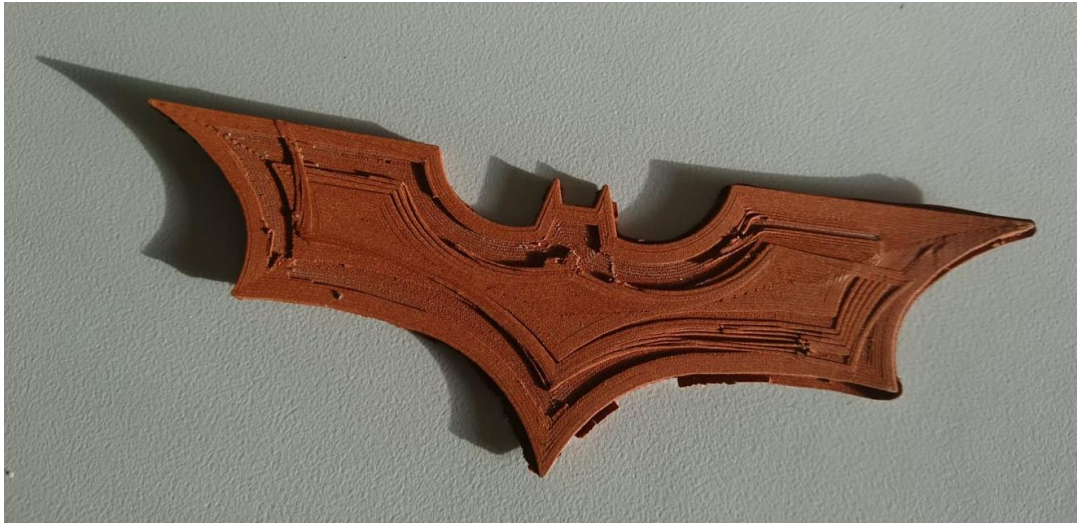
Figure 46 - Upper view of FDMet produced copper part with complex geometry
