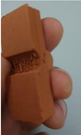
Figure 37 - View of a FDMet produced copper part with a conformal channel
