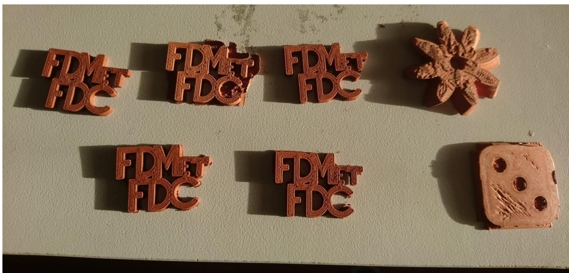
Figure 47 - FDMet produced copper parts with complex geometry
