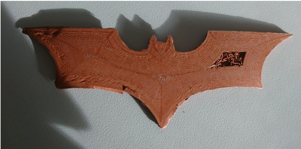
Figure 45 - Bottom view of FDMet produced copper part with complex geometry
