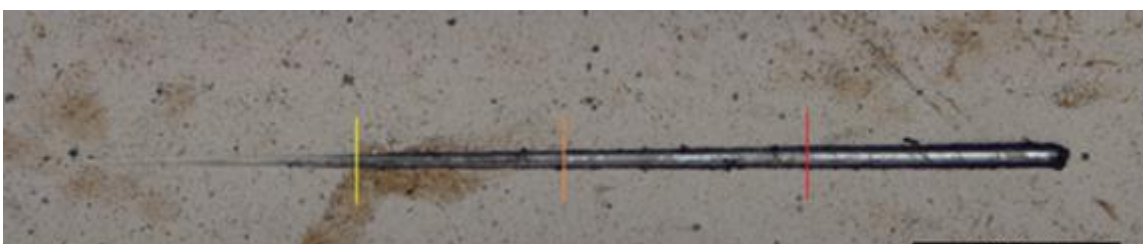
Figure 4.7 Scratch test on W-DLC with the identification of the zones of cohesive failures (yellow) and adhesive failures (orange and red) being the red one indicative of the delamination zone of the coating from the substrate.
