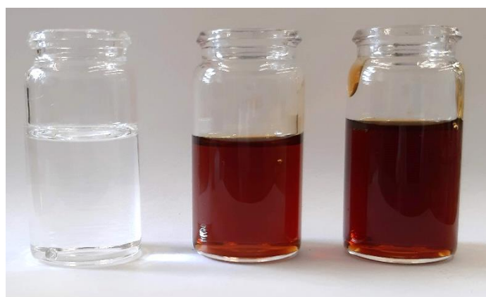
Figure 4.10. Lact:Tart:ChCl (4:1:1) before use (left), after 1 extraction process (middle) and after 2 extraction cycles (right).
