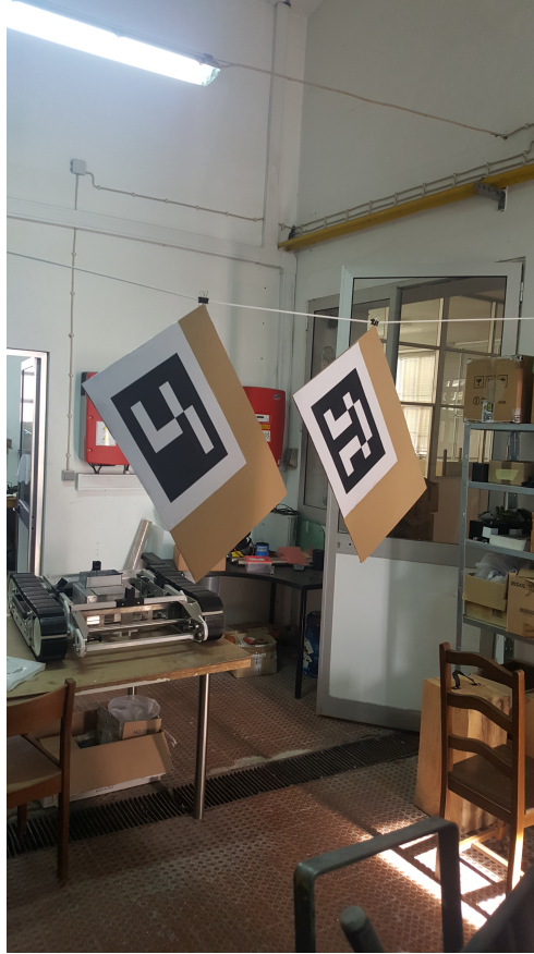
Figure 4.1: Setup used to calibrate the Intel D435 camera with the 3D LIDAR. It was set up inside a room where there is no wind interference so the boards remain static throughout the calibration process.
