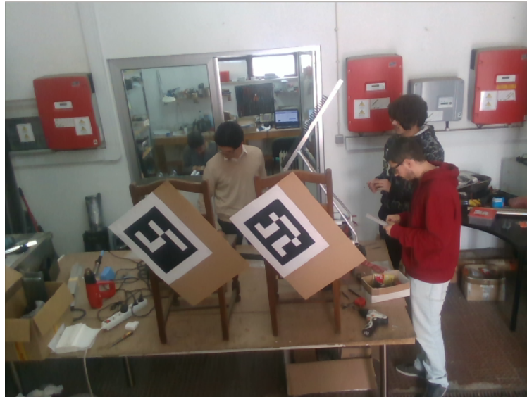
Figure 4.10: Setup for LIDAR-Stereo camera registration validation.
