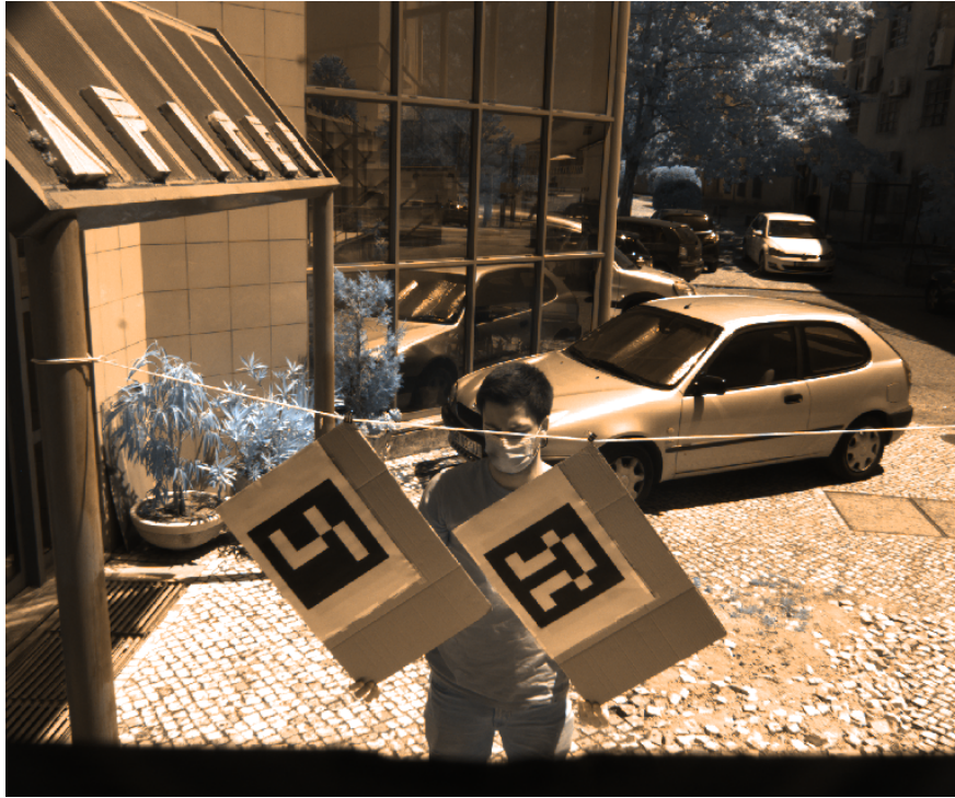
Figure 4.3: Setup used to calibrate the multispectral (monocular) camera with 3D LIDAR. It is similar to the setup used for stereo cameras but ArUcos are now a key agent for calibration. Human intervention was required to keep the boards static because the test was done in a moderately windy environment.
