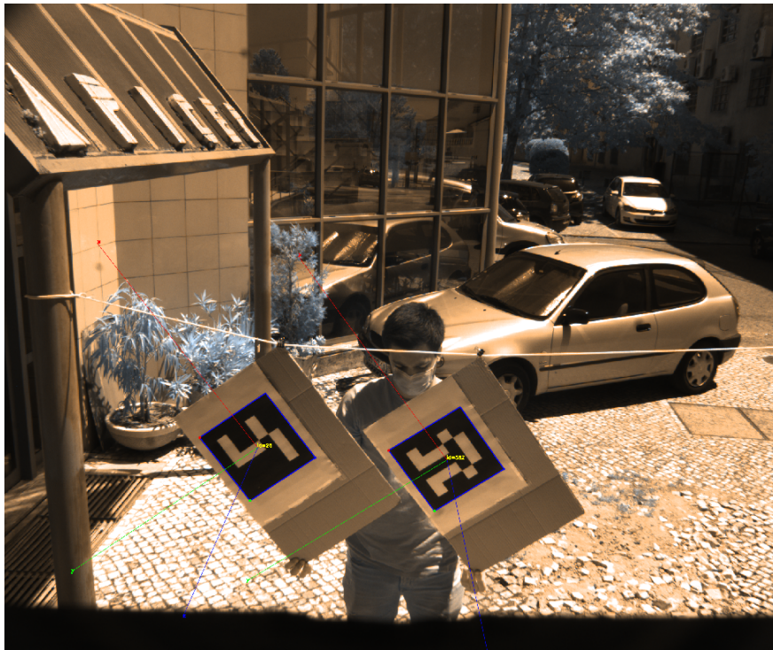
Figure 4.4: Detection of ArUco markers. It is possible to know the center of the marker, an axis that represents the plane that includes each pair of markers with their board, the marker ID and even an outline of the marker format.
