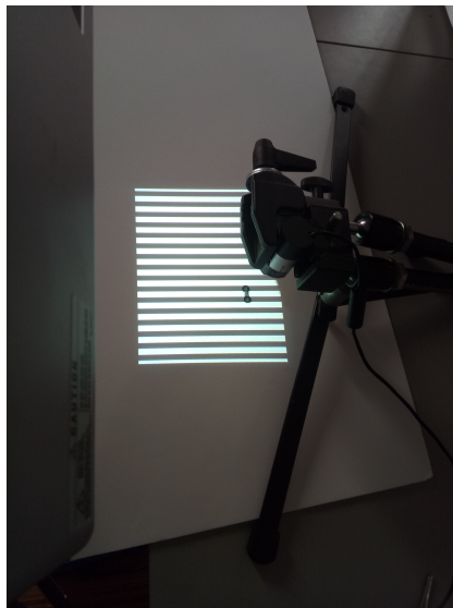
Figure 3.3: Structured Light System composed of a camera and a projector.
