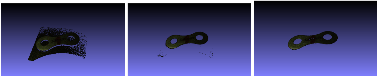
Figure 4.9: Left: Reconstruction of the scene; Middle: Plane removed from the scene; Right: Point cloud after applying the SOR filter
