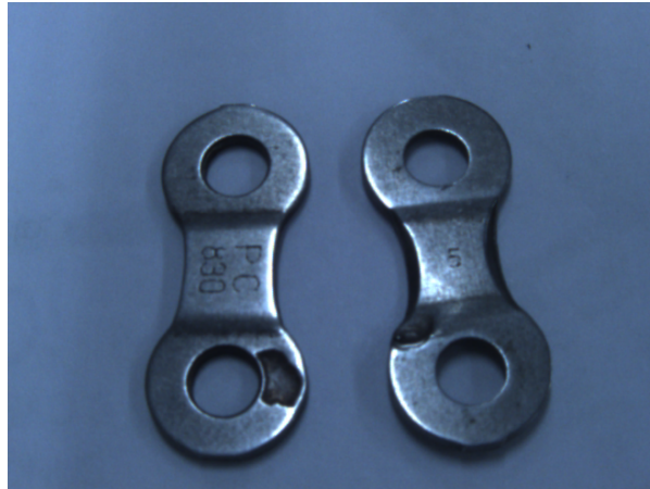
Figure 1.3: Examples of surface defects (1.I)
