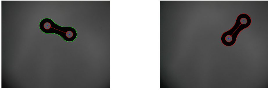
Figure 4.5: Left: The system incorrectly measures the size of the holes and the distance between them; Right: System incorrectly measures every parameter.
