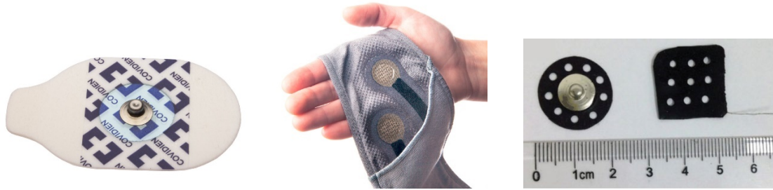
Figure 8 – a) The conventional Ag-AgCl electrodes used in this project [22]; b) The Nuubo wearable ECG sensor [23], based on textile electrodes to increase durability and comfort; c) CNT based electrodes promise small footprint and very high durability [24].
