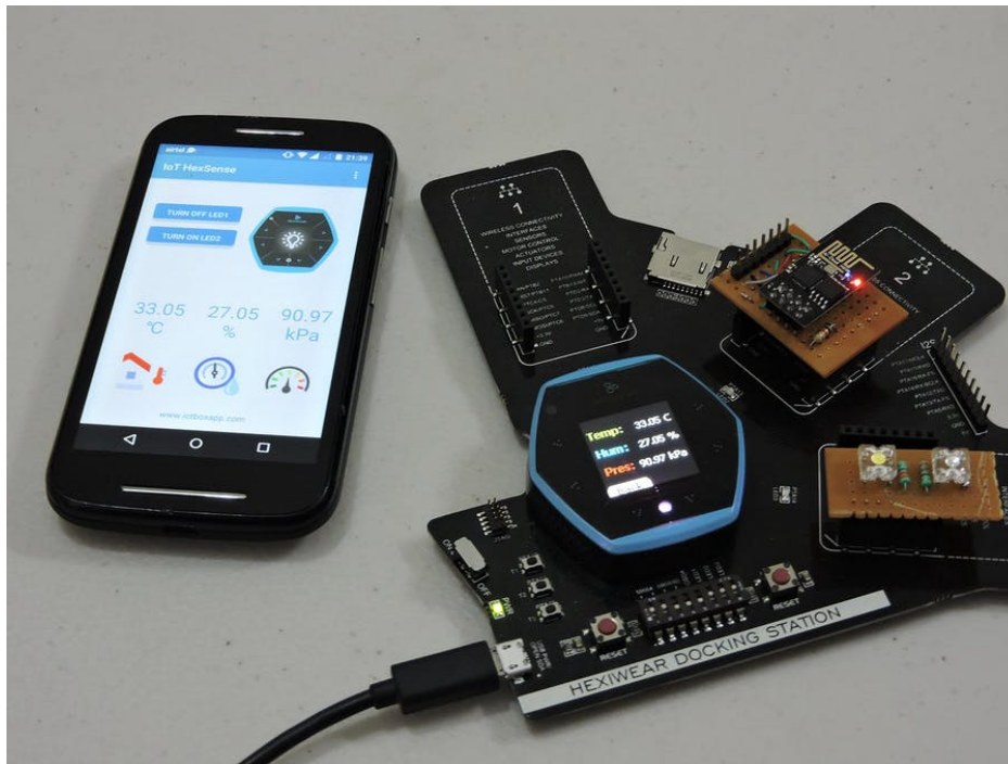
Figure 14 – The Hexiwear system in its docking station with two custom made clickboards plugged in. It has wireless connectivity with the smartphone and a small OLED display. Requires the docking station for expandability [35].
