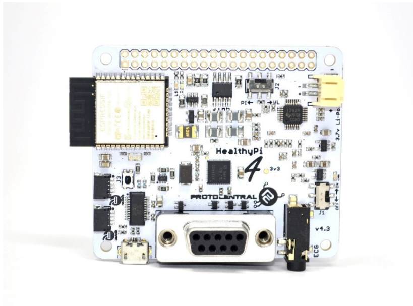
Figure 16 – The HealthyPi hat comes in a Raspberry Pi “Hat” form factor but can also be used standalone with a battery connected (top right). It includes I/O for a pulse oxymeter (RS232 9 pin) and ECG (3.5 mm) sensors as well as BLE and Wi-Fi communication [37].
