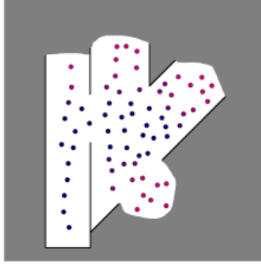
Figure 2.4: Representation of the cached nodes in the map using the potential information gain [10].
