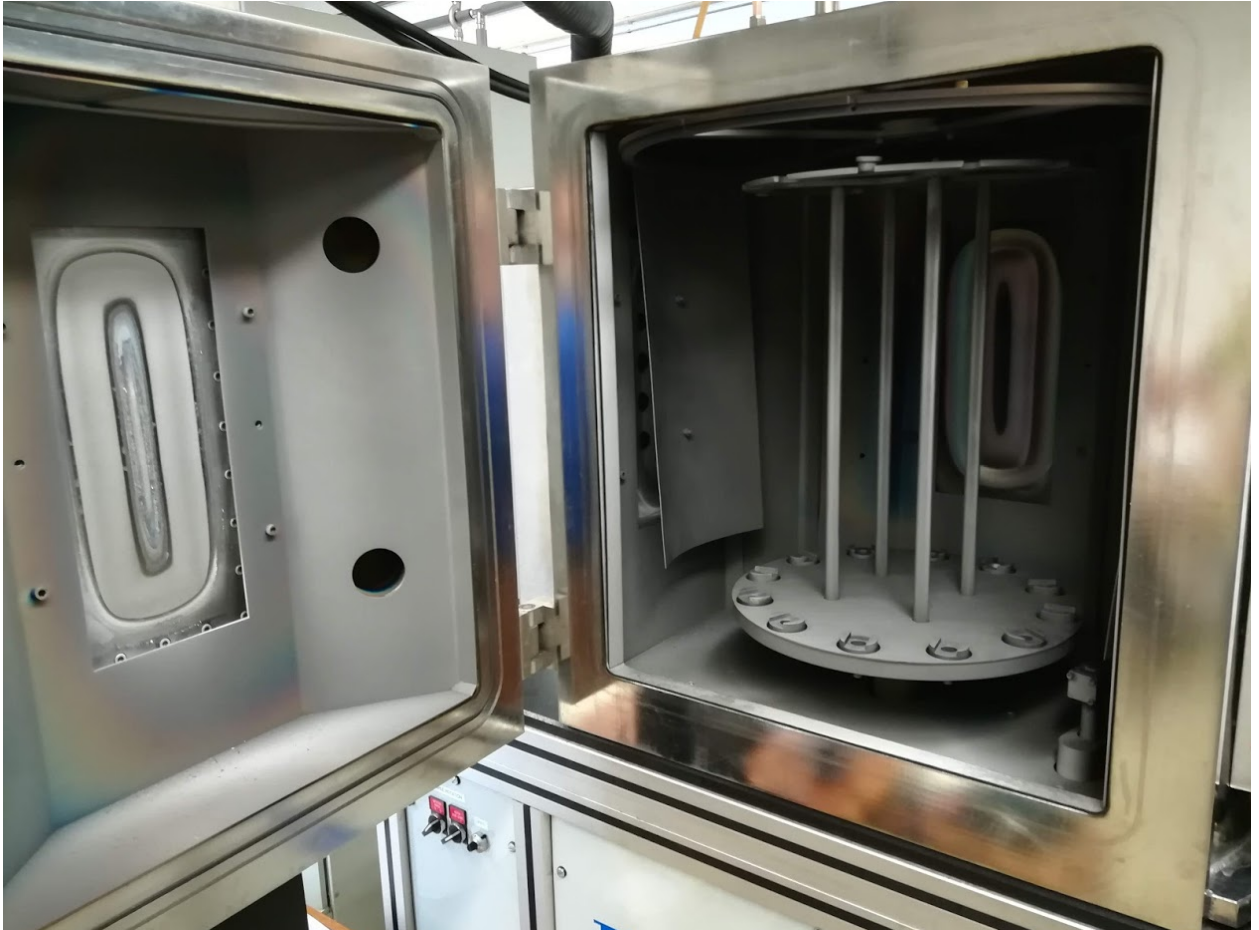
Figure 3-3 Teer UDP 650/4 deposition unit
