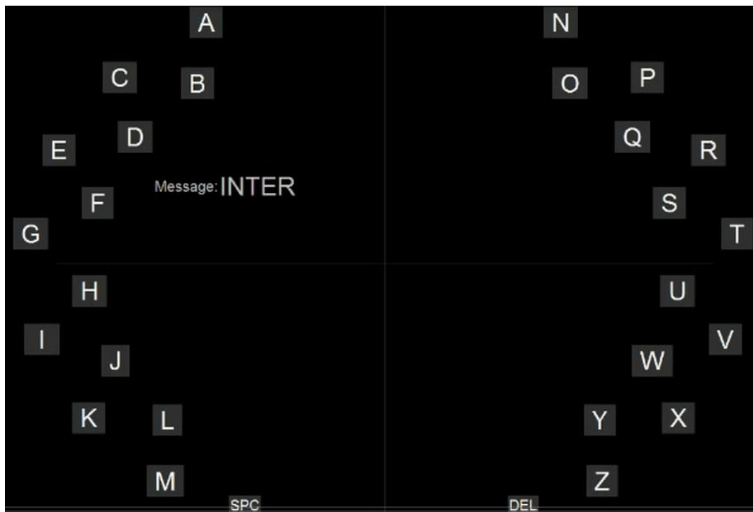
Figure A.1: Lateral single character speller paradigm [Cruz et al., 2018a]. Each symbol is highlighted once in each round. The highlight time of the stimuli is 75 ms and the inter-trial interval is 4s.
