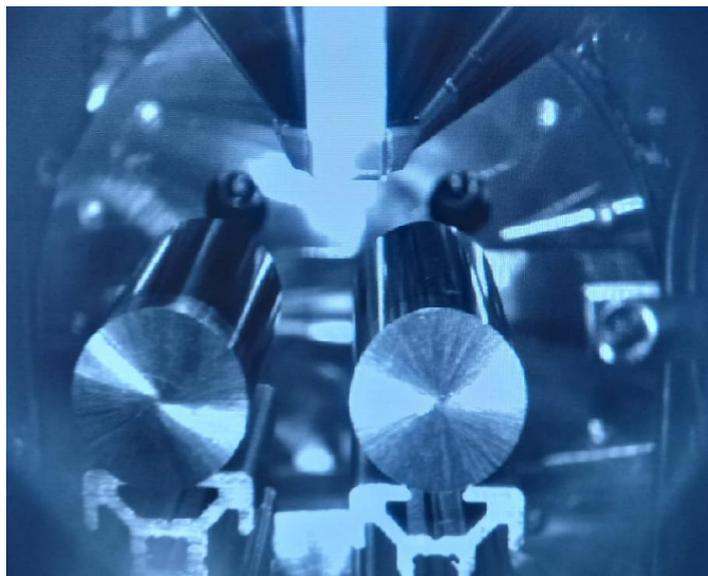
*Figure 19 Cylindrical sample holder used for analysis in SEM*
