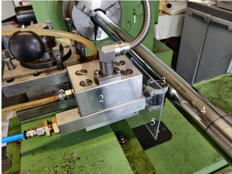
*Figure 18 Experimental Setup: Mechanical lathe (1), Dynamometer (2), Coated cylinder (3), Counter cylinder (4), and transparent panel to block the air (5)*
