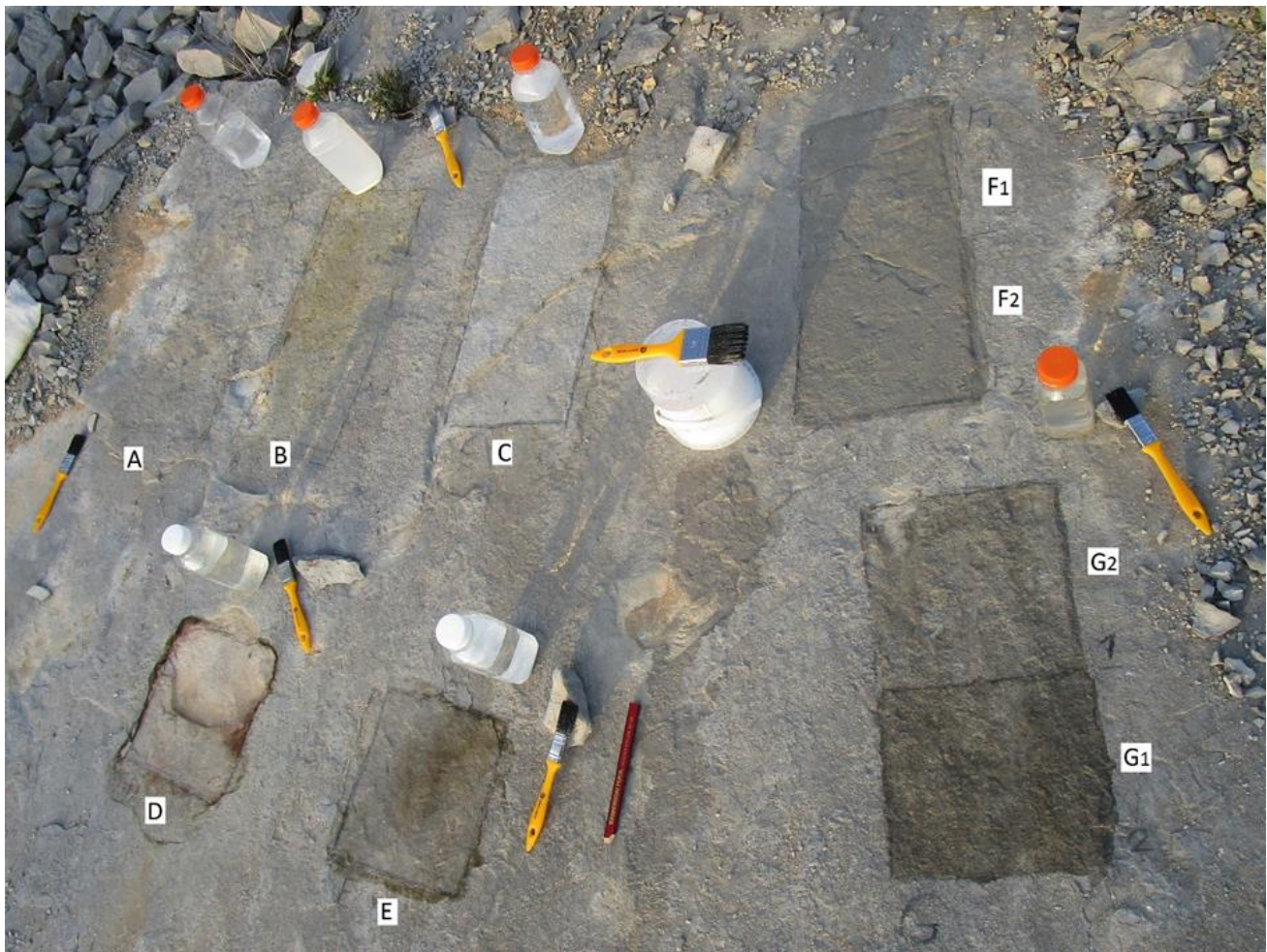
Figure 7. Long-term experiment with application of various products for limestone surface stabilization to weathering in a selected area of Bed 5 bedding plane at Cabeço da Ladeira fossil site: (A) lime water (aq.); (B) barium hydroxide (aq.); (C) ammonium oxalate (aq.); (D) solution of barium hydroxide in ethanol; (E) ammonium oxalate solution in ethanol; (F) nanosilica (upper half—F1—one coating layer, lower half—F2—two coating layers); and (G) paraloid B-72 solution in ethanol (upper half—G1—one coating layer, lower half—G2—two coating layers). Dimensions of the areas where the products were applied: 20 \times 40 cm and 20 \times 20 cm.
