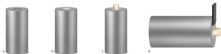
Figure 1. Schematic diagram of the experiment set-up showing how the samples were prepared for SBS strength testing: (a) cylindrical metallic blocks; (b) the hole in the middle was filled with the CSC; (c) after adhesive procedures, a sectioned gelatin capsule was applied on the surface of the CSC and filled with the flowable composite resin; (d) a chisel-edge plunger was mounted into the testing machine and positioned, so that the leading edge was aimed at the CSC/adhesive interface. Adapted from Altunsoy, Tanriver, et al. and from Palma et al. [10,11].
