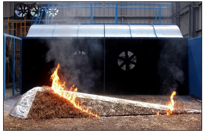
Fig. 5. Image showing the hill model placed in the combustion wind tunnel during one of the experiments, the rounded end is attached to the left side of the model.
