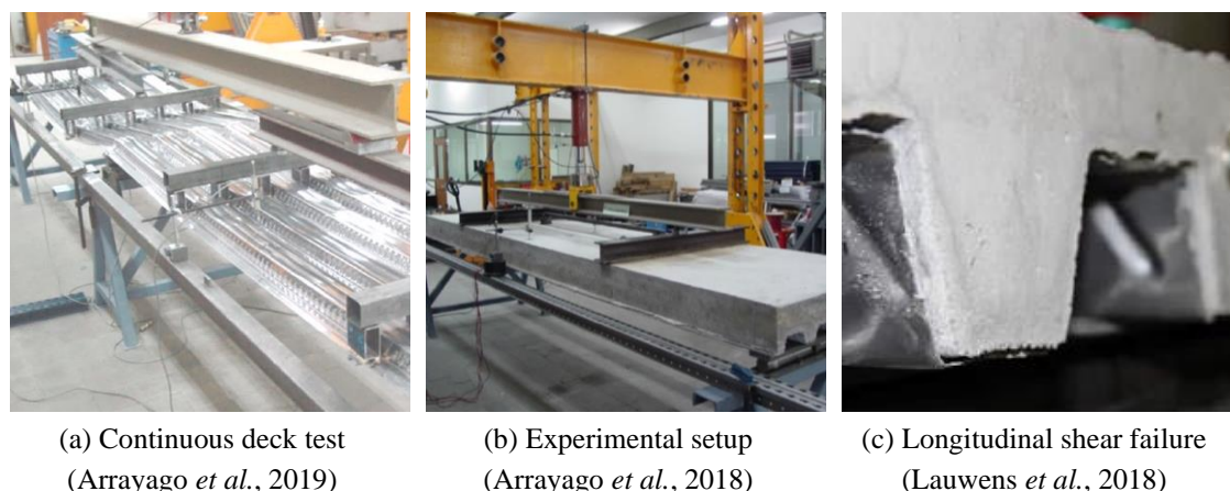
Fig. 2.21 Experimental tests on composite slabs with ferritic stainless steel decks
