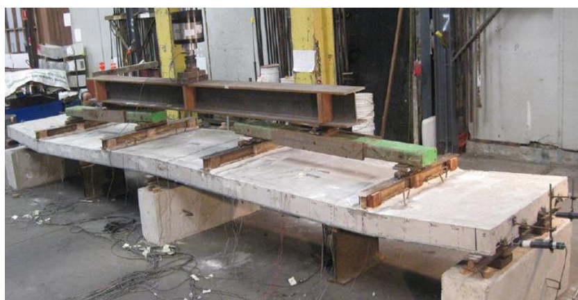
Fig. 2.4 Bending test to continuous composite slabs (Gholamhoseini, 2018)
