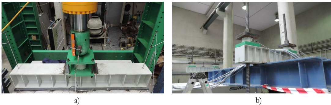
Fig. 6.11: Test setup: a) load application; b) end support - 2 back-to-back U260 beams (white) and 2 HEB300 beams (blue)
