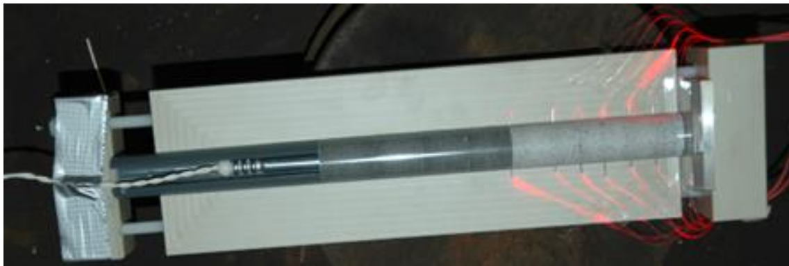
Figure 4-4: Pellets explosive charge where the darker pellets are HWC and the lighter are TKX-50.
