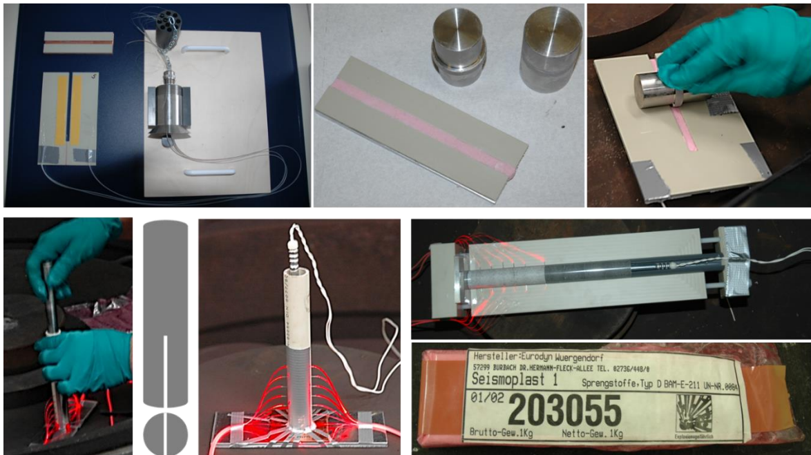
Figure 3-2: Sample container, “U” plate, detonation port, and probes transport bucket ready to take to the detonation chamber (top left). Tools specially designed for the insertion of Seismoplast into the RECs and half REC assembled (top middle). Insertion of Seismoplast in the “U” plate (top right). Insertion of Seismoplast in a CEC with a tool specially designed for it and its scheme with the lateral and bottom view (bottom left). Assembled CEC charge for D and U_s measurements with OAM (bottom middle). A PEC assembled with HWC (dark gray) and TKX-50 (light gray) for measurement of the D of TKX-50 and U_s (middle right) and a package of Seismoplast (bottom right).
