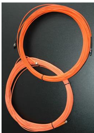
Figure 3-4: 25 m step-index multimode fiber optic patch cables and their spectral attenuation (in blue). Graph from (THORLABS, 2019)
