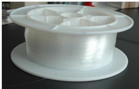
Figure 3-3: A spool of PMMA optical fiber and its spectral attenuation. Graph from (Laser Components, 2016)
