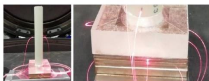
Figure 2. Complete sample assembly (left) and zoomed image (right) of a configuration 1 prepared to characterize the shock wave velocity in Cu. The PMMA block, above the Cu stack, worked as a charge holder. The active optical probes are conducting the red laser radiation.
