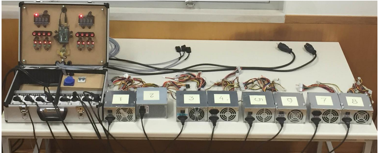
Figure 3.9 - Setup for ageing the DUTs using the platform created
