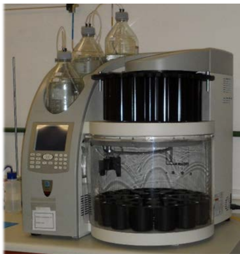
Figure III.9. Dionex® ASE 350 extraction equipment.
