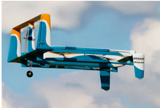
Figure 4: A Fixed Wing Hybrid drone (from [14]).
