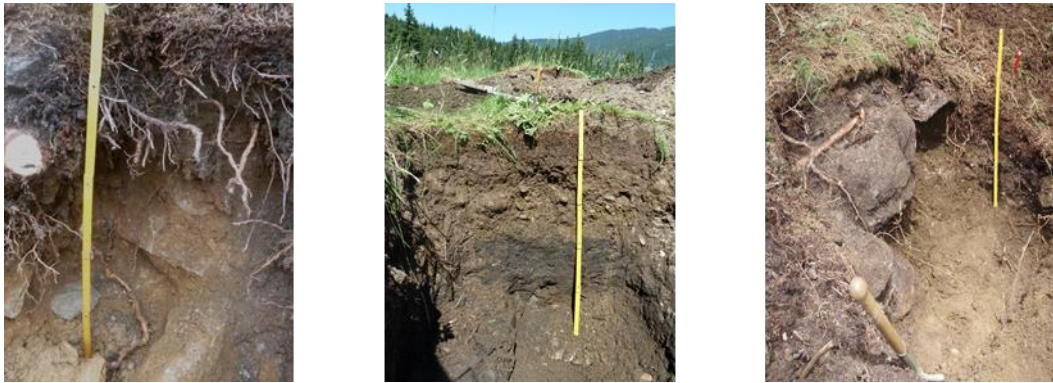
Fig. 2.6. Large representative elementary volumes at field sites taken for rock fragments content measurement in stony soils (Photographs taken by the Institute of Hydrology, Slovakia research team).
