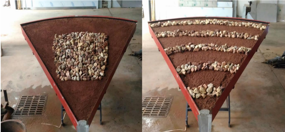
Fig. 2.4. Different distribution patterns of 50% surface rock fragments cover on a converging plane soil surface in controlled laboratory conditions (Photographs taken by the author of this thesis on the 10th June, 2017).
