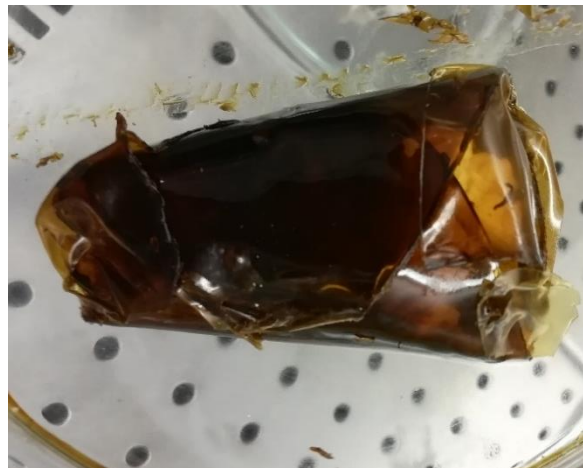
Figure 11 Latin-style fresh cheese wrapped with the whey protein-based edible film incorporated with the green tea extract.
