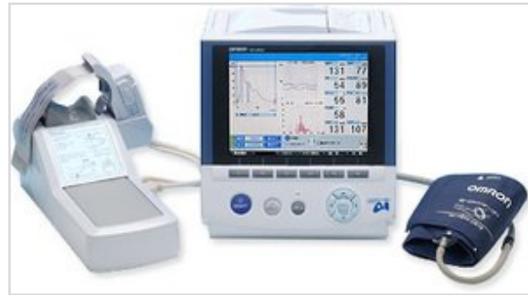
Figure 10. HEM 9000ai® system. From left to right: A/x pulse wave measurement unit, main unit and cuff. Adapted from [26].
