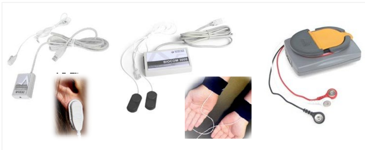
Figure 16. HRVlive® hardware. Adapted from [32]. (a) Biocom HRM-02 pulse wave sensor; (b) Biocom 3000 ECG recorder; (c) Active ECG recorder®.
