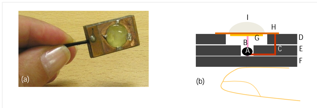
Figure 24. Final PZ probe. (a) Photo; (b) cross scheme; A – coaxial Cable; B – PZ signal conductor; C – ground conductor; D – perforated plate; E – perforated plate (small perforation); F – plate with no perforation; G – PZ material; H – metal disk; I – silicone rubber.
