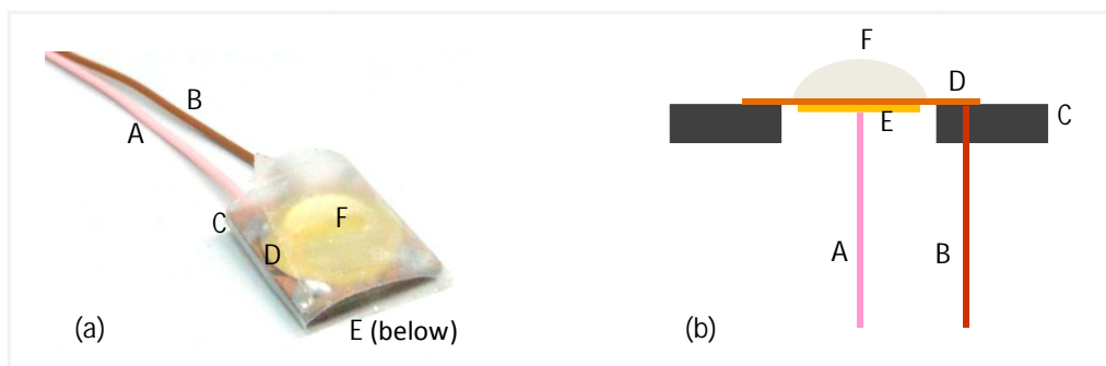
Figure 23. Initial PZ probe. (a) Photo; (b) cross scheme; A and B – signal and ground connectors; C – PCB; D – metal disk; E – PZ material; F – silicone interface.
