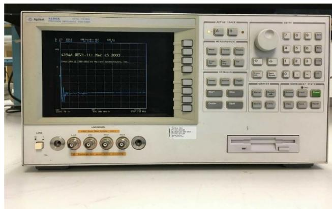
**Figure II.15** : Agilent 4294 A Precision impedance Analyzer
