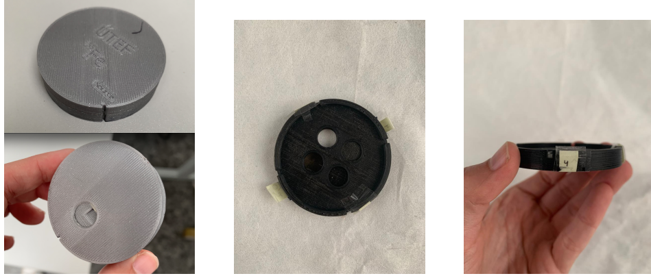
FIGURE 4.16: Source and masks used in the thickness test. Left: ^{55}\text{Fe} source used in the laboratory. From the top and from the bottom. Centre: Picture of the mask from the top. Right: Picture of the mask from the side.
