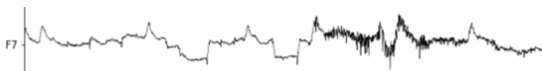
Figure 8: Example of artifact produced by muscle activity in EEG data (Extracted from [42]).
