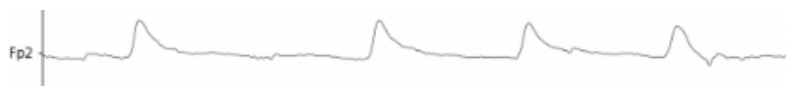
Figure 6: Example of artifacts introduced by eye blinks in EEG data (Extracted from [42]).
