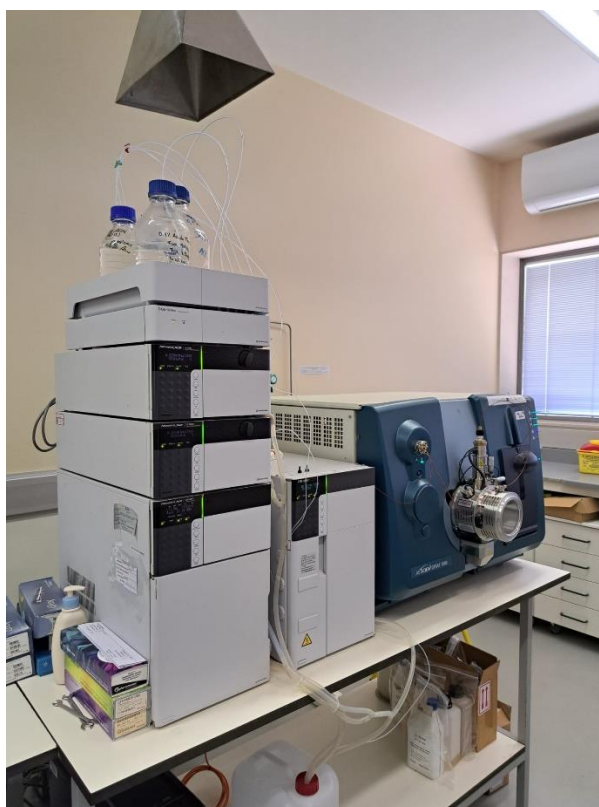
Figure 15. UHPLC-MS/MS equipment at INIAV, I.P. facilities (Vairão campus, Vila do Conde).
