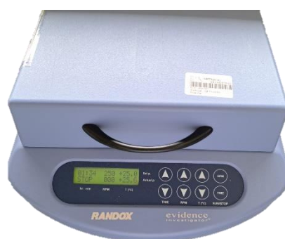
Figure 4. Photography of the thermoshaker used to incubate the carriers.
